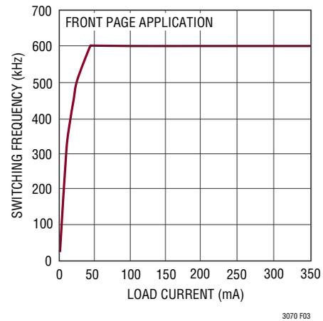
Figure 3. Switching Frequency in Burst Mode Operation
