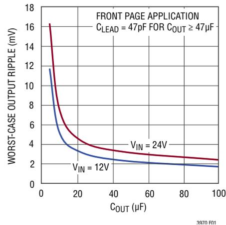
Figure 1. Worst-Case Output Ripple Across Full Load Range
