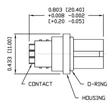
MATERIAL HOUSING: PBT UL94V-0, BLACK CONTACT: BRASS BRASS NUT: **EPDM** □-RING: **FINISH** CONTACT: GOLD PLATED □VER 504" NICKEL NUT: NICKEL PLATED 60u" TO 10u" OVER ALL ELECTRICAL RATED CURRENT: 4A 60V RATED VOLTAGE: INSULATION RESISTANCE: 100 MOhms MIN. CONTACT RESISTANCE: 10 mOhms MAX. WATER PROOF: IP67 **ENVIRONMENT OPERATION TEMPERATURE:** -40°C TD +85°C MAX WIRE AWG: 22
