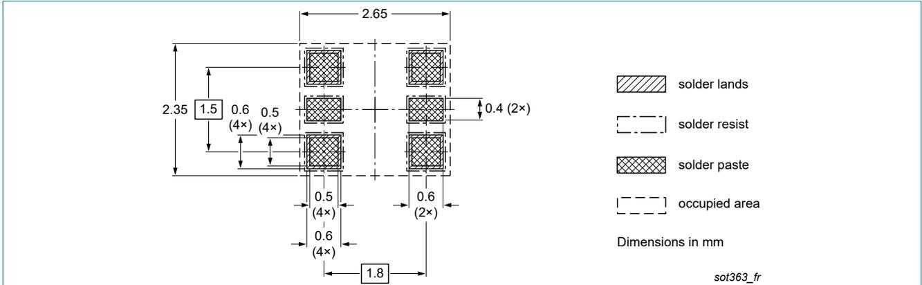
Fig. 11. Reflow soldering footprint for TSSOP6 (SOT363)
