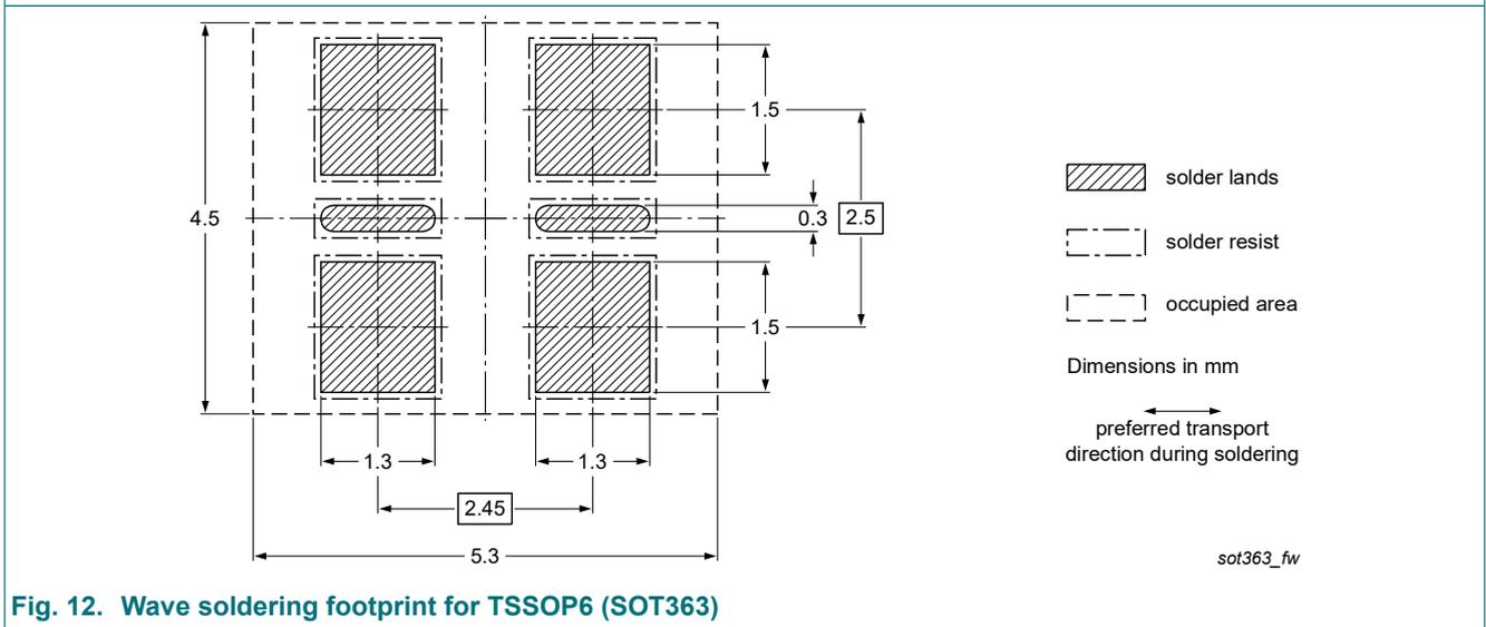
Fig. 12. Wave soldering footprint for TSSOP6 (SOT363)
