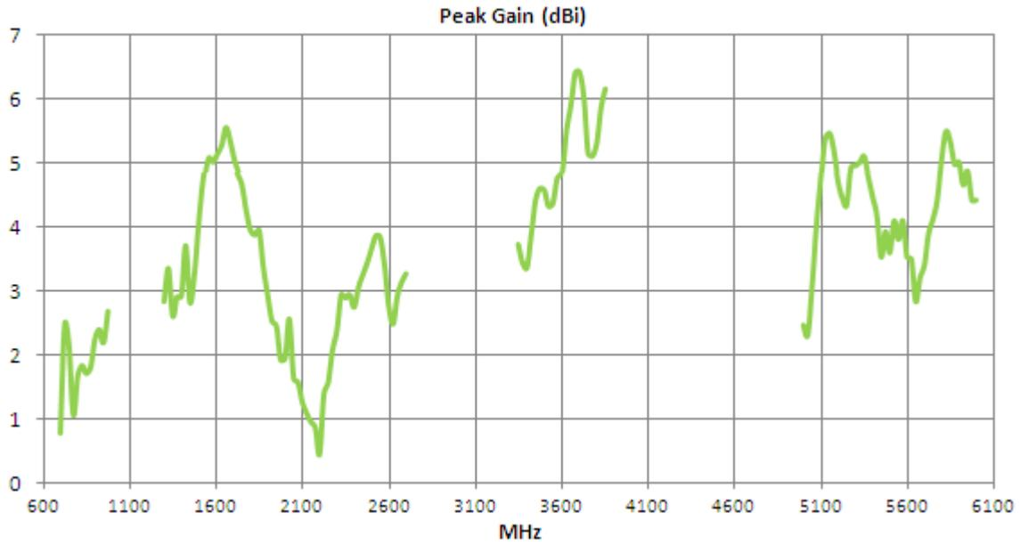
Figure 5. Peak Gain of FXUB66 UWB Antenna.
