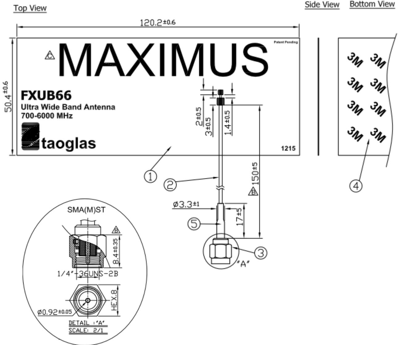
**Figure 20.** Mechanical drawing of FXUB66 UWB Antenna.
