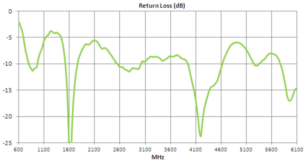
**Figure 2.** Return loss of FXUB66 UWB Antenna.
