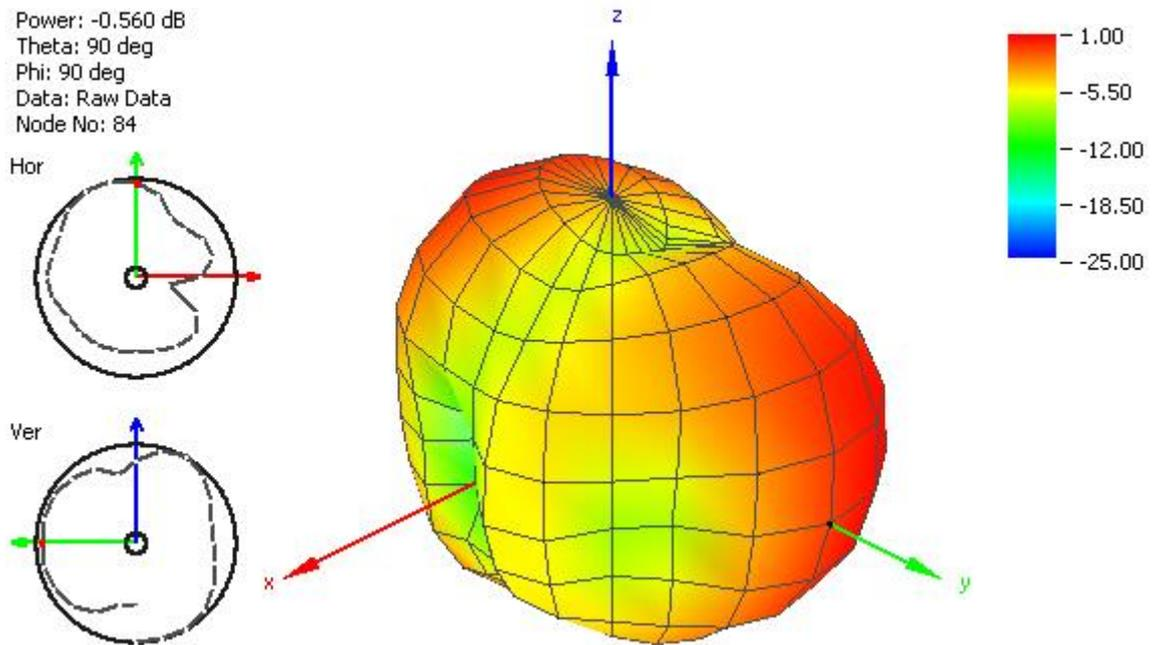
**Figure 15.** Radiation Pattern at 2100 MHz of FXUB66 UWB Antenna.
