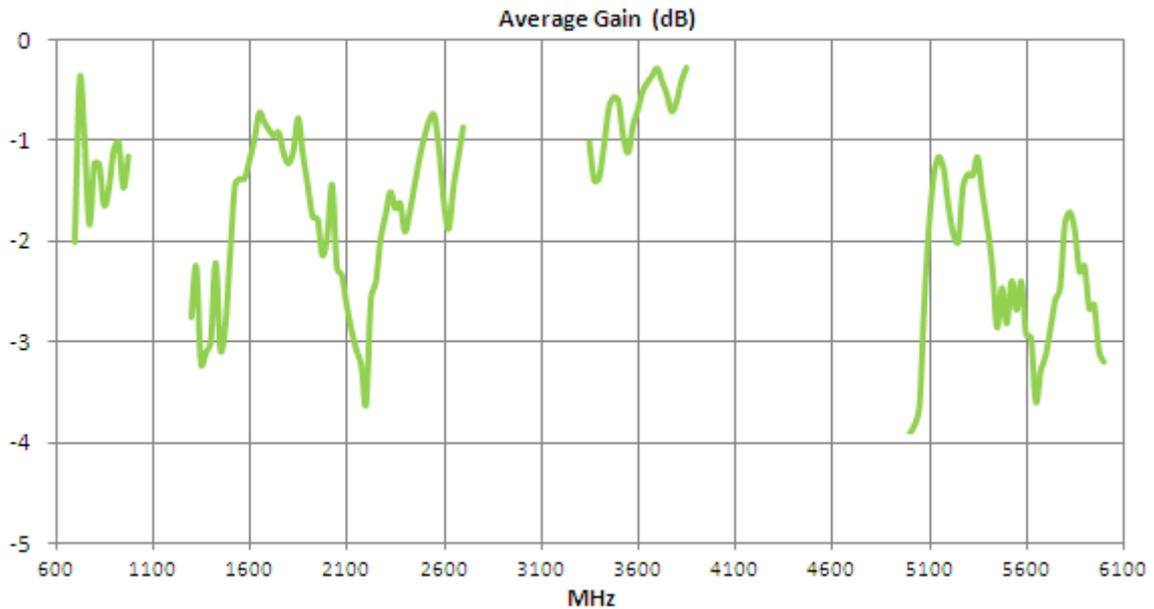
Figure 6. Average Gain of FXUB66 UWB Antenna.
