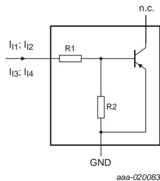
Fig 32. Resistor test circuit
