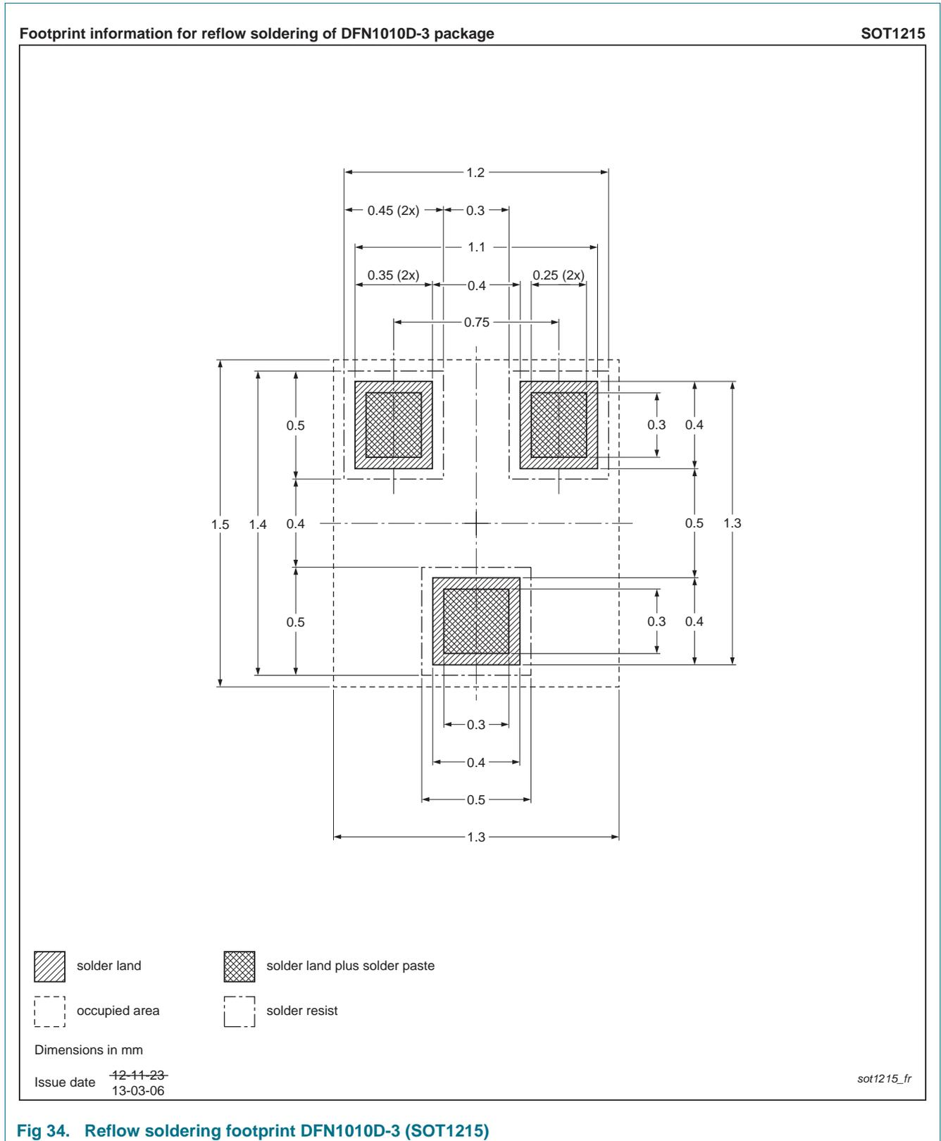
Fig 34. Reflow soldering footprint DFN1010D-3 (SOT1215)
