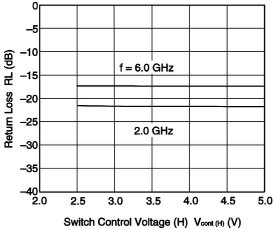
RF1/RF2 RETURN LOSS vs. SWITCH CONTROL VOLTAGE (H)
