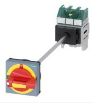
SENTRON, Molded case switch 3LD5 UL, Emergency switching-off, 3-pole, certified according to UL489 UL60947-4-1 and IEC60947-3, UL: 30A, SCCR 50kA at 480VAC, Operating power at 480VAC 3-phase: 20hp, IEC: 32A, Operating power at AC-23A at 400V: 15kW, floor mounting with door coupling rotary operating mechanism, defeatable, emergency switching 4-hole mounting of the handle, without tolerance compensation, incl. terminal covers for the infeed side
