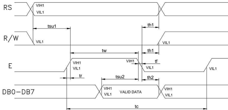
Read cycle ( $T_a=25^\circ\text{C}$ ,  $V_{DD}=5.0\text{V}$ )
