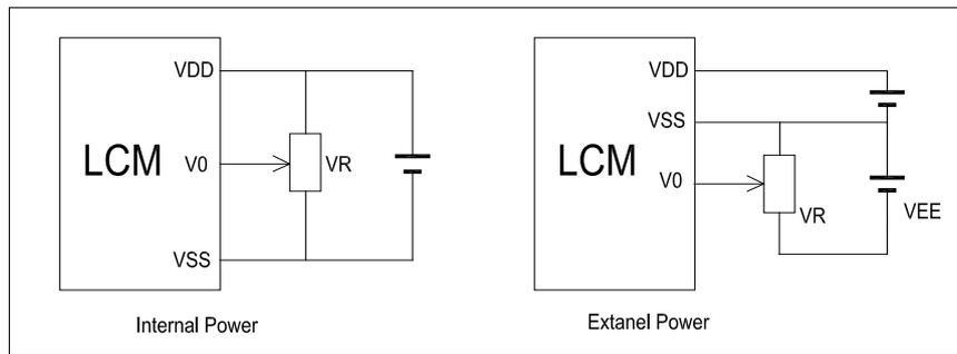
VDD~V0: LCD Driving voltage
