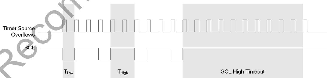
**Figure 24.4. Typical SMBus SCL Generation**
