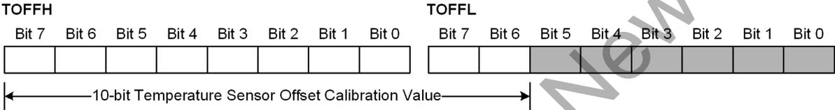
Figure 9.2. TOFFH and TOFFL Calibration Value Orientation
