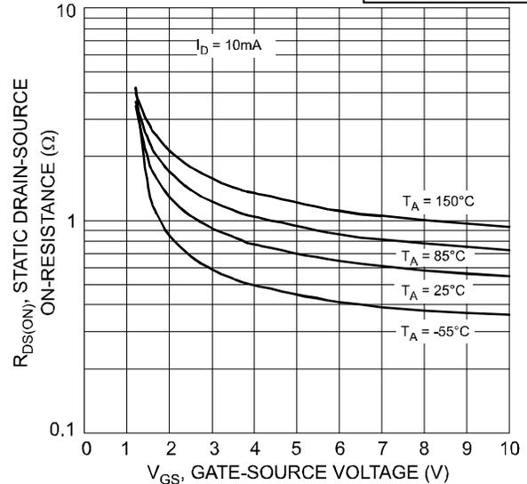
Fig. 4 Static Drain-Source On-Resistance vs. Gate-Source Voltage
