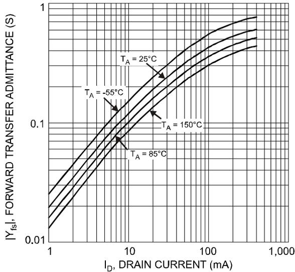
Fig. 9 Forward Transfer Admittance vs. Drain Current
