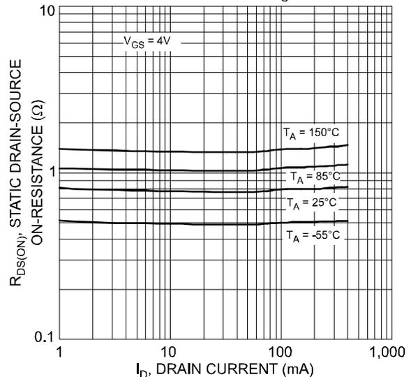
Fig. 6 Static Drain-Source On-Resistance vs. Drain Current
