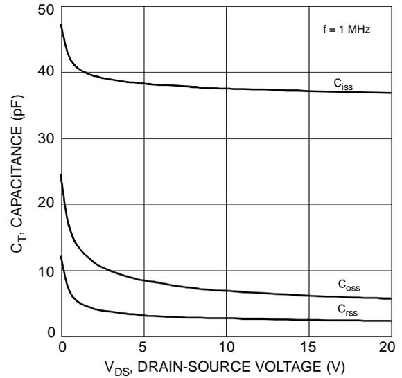
Fig. 10 Typical Capacitance
