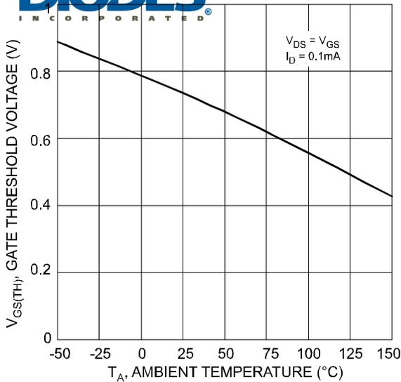
Fig. 3 Gate Threshold Voltage vs. Ambient Temperature
