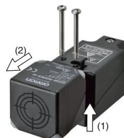
3. When positioning the sensing surface to the side, rotate it to the required position, then fit it into the case. (The possible positions are 0, 90, 180, and 270°. Do not forcefully rotate the sensing surface.)
