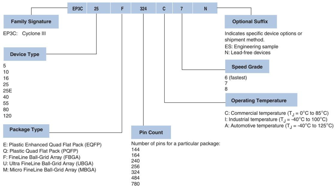
**Figure 1-2.** Cyclone III LS Device Packaging Ordering Information
