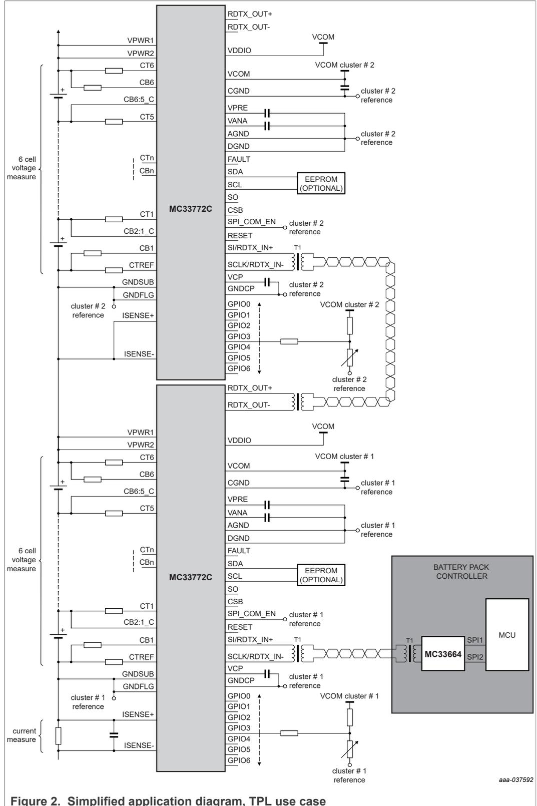
Figure 2. Simplified application diagram, TPL use case
