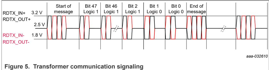
Figure 5. Transformer communication signaling
