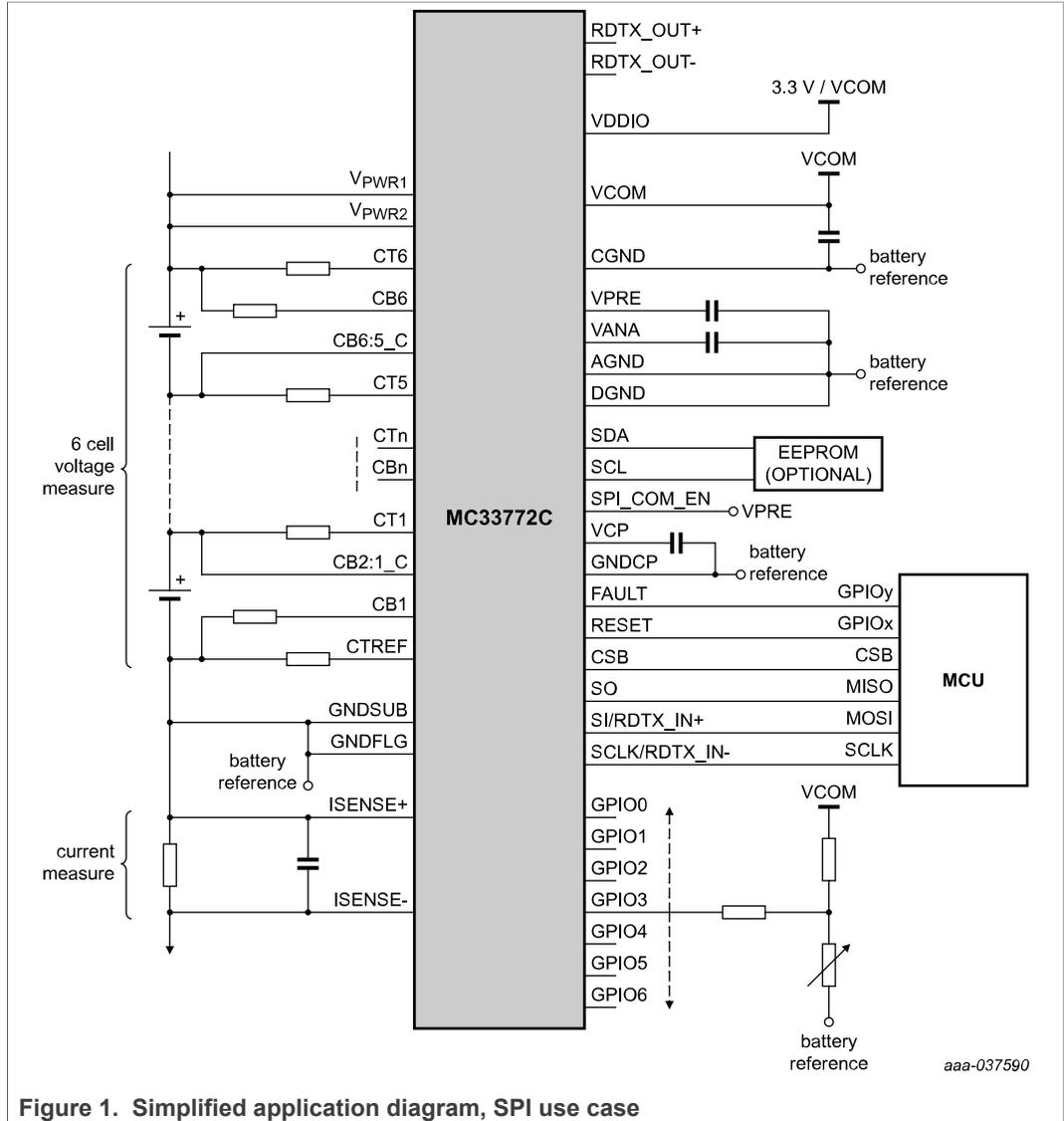
Figure 1. Simplified application diagram, SPI use case
