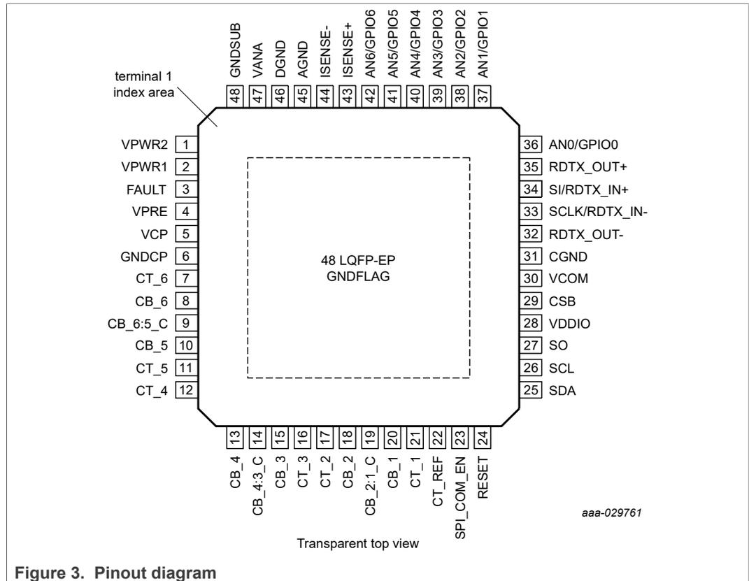
Figure 3. Pinout diagram
