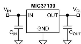
Figure 1. Capacitor Requirements
