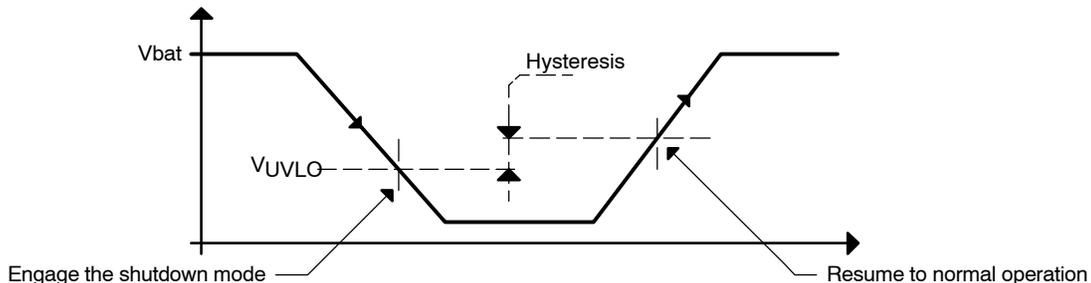
Figure 22. Undervoltage Lockout Basic Mechanism
