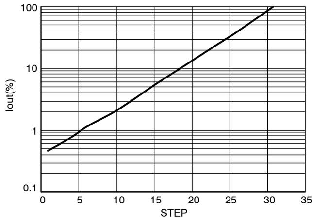
**Figure 10. Typical Iout (%) versus ILED Step Value**
