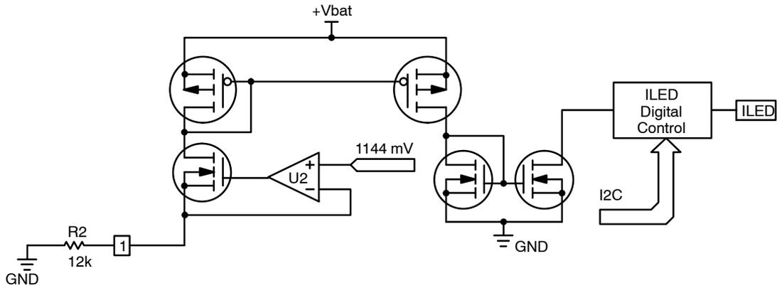
**Figure 9. Basic Reference Current Source**
