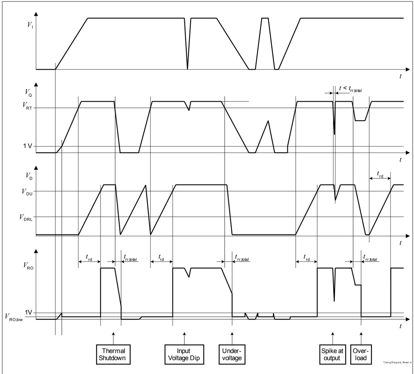
**Figure 6** Timing diagram reset
