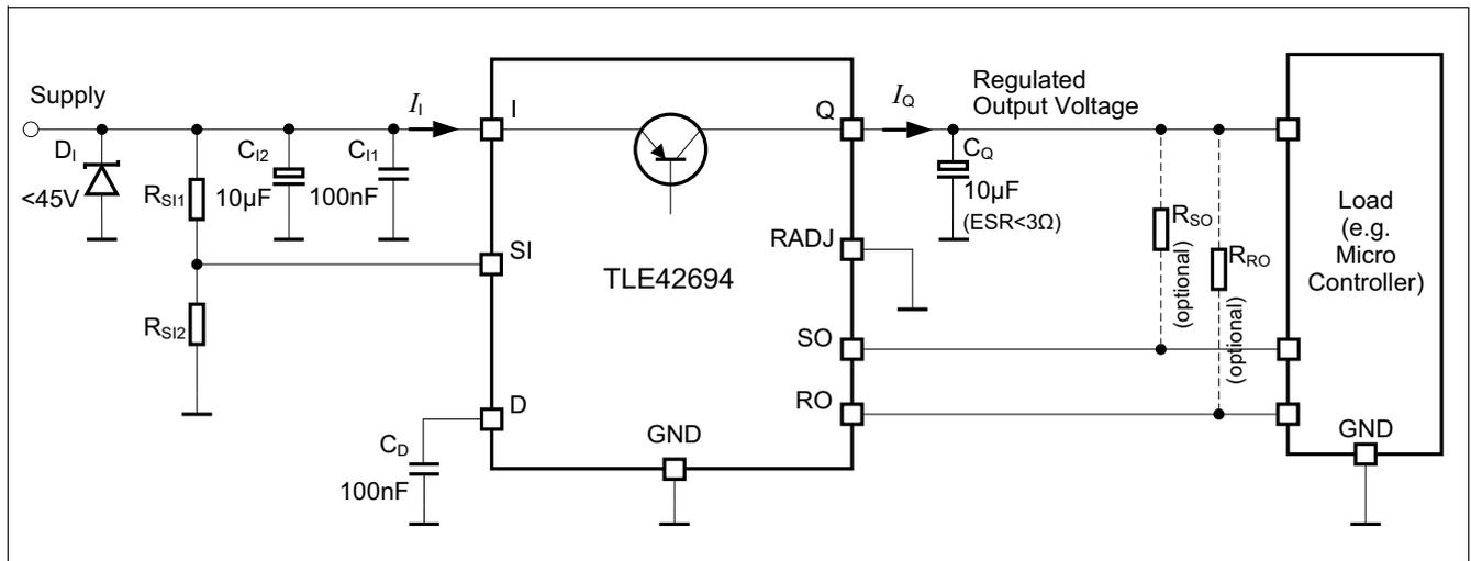
**Figure 8 Application diagram with selecting default reset thresholds**
