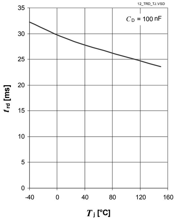
**Power-on reset delay time  $t_{rd}$
