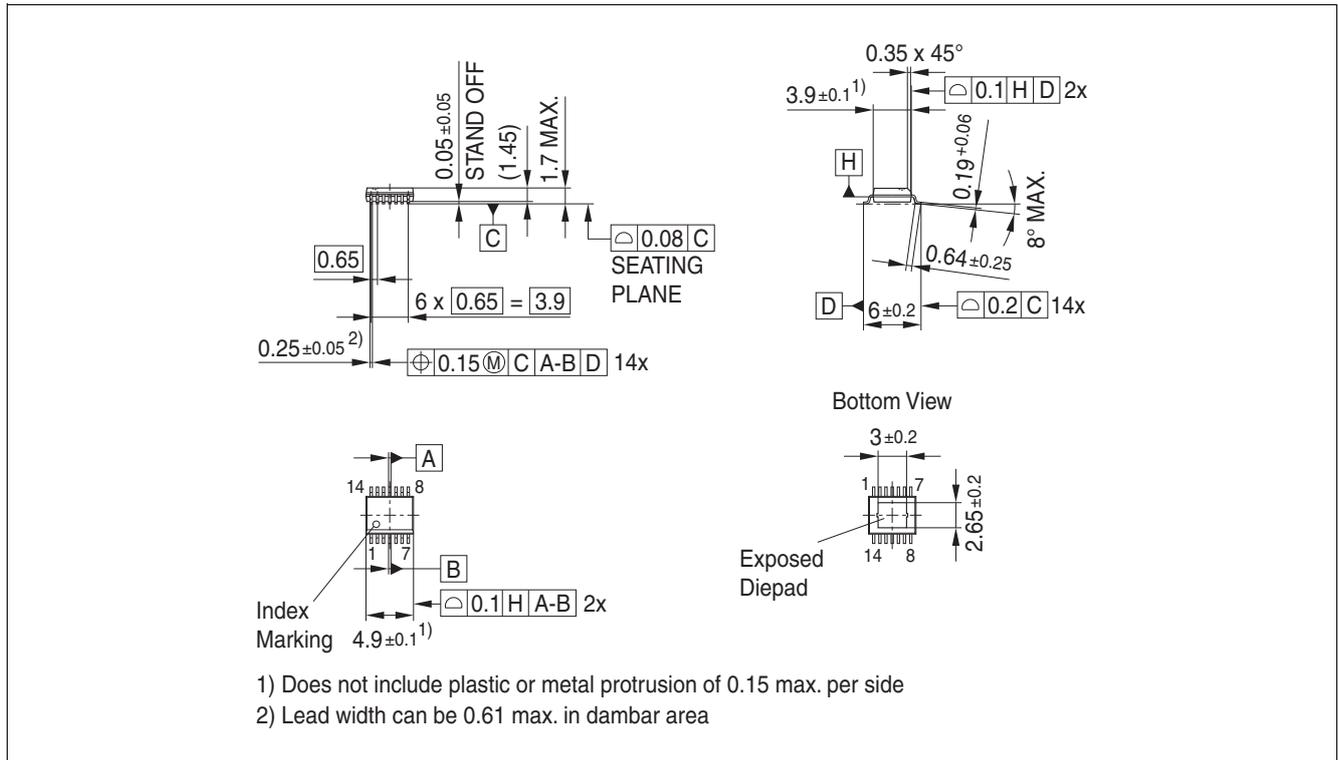
**Figure 12 PG-SSOP-14 exposed pad<sup>1)</sup>**
