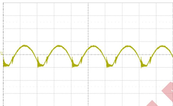
Fig. 15: Input reflected ripple current,  $i_c$  (1 A/div.), measured at input terminals at full rated load current and  $V_{in} = 48 \text{ V}$ . Refer to Fig. 14 for test setup. Time scale:  $2 \mu\text{s}/\text{div}$ .
