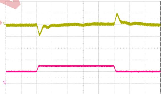
Fig. 10: Turn-on transient at full rated load current (resistive) plus 4700  $\mu\text{F}$  at  $V_{in} = 48\text{ V}$ , triggered via ON/OFF pin. Top trace: ON/OFF signal (5 V/div.). Bottom trace: output voltage (5 V/div.). Time scale: 20 ms/div.
