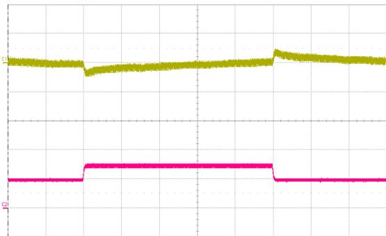
Fig. 13: Output voltage ripple (50 mV/div.) at full rated load current into a resistive load with  $C_o = 10 \mu\text{F}$  tantalum +  $1 \mu\text{F}$  ceramic and  $V_{in} = 48 \text{ V}$ . Time scale:  $2 \mu\text{s}/\text{div}$ .
