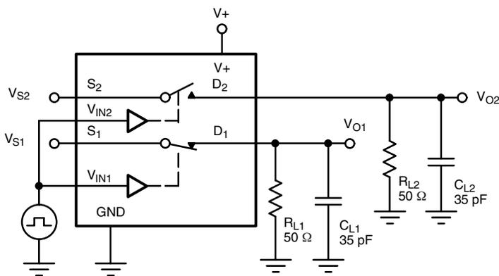
$C_L$  (includes fixture and stray capacitance)
