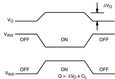
**Figure 3. Charge Injection**
