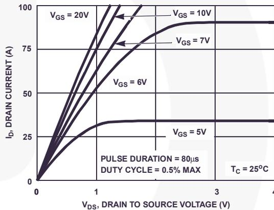
**Figure 8. Saturation Characteristics**
