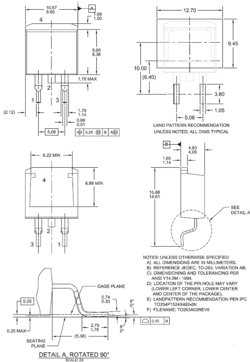
**Figure 22. TO263 (D<sup>2</sup>PAK), Molded, 2-Lead, Surface Mount**
