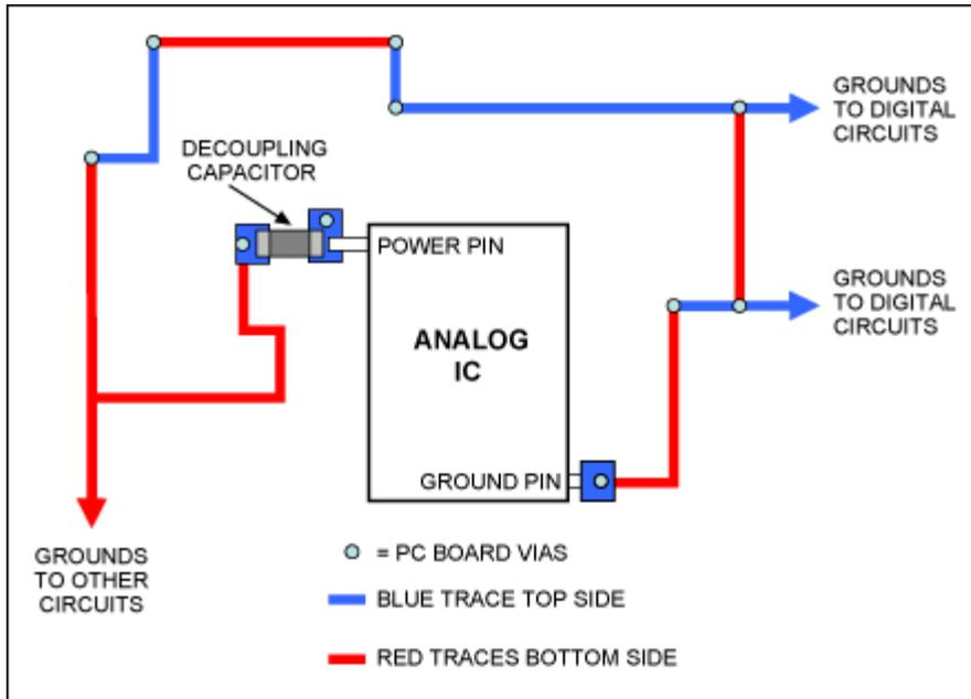
Figure 2. Board layout viewed using the PCB design software.
