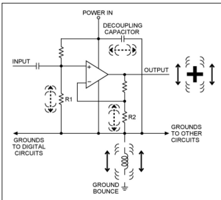
Figure 3. A way to visualize ground bounce in the circuit.
