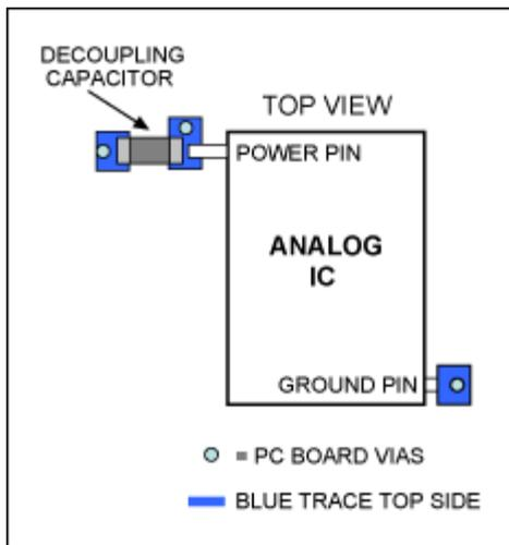
Figure 1. A printed circuit board (PCB) layout showing IC and capacitor.
