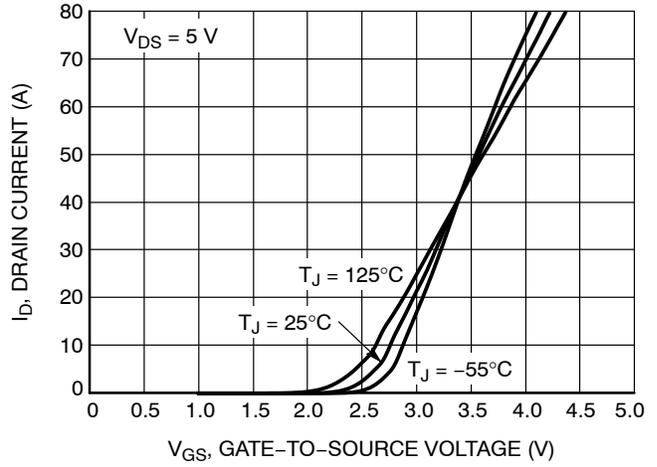
Figure 2. Transfer Characteristics
