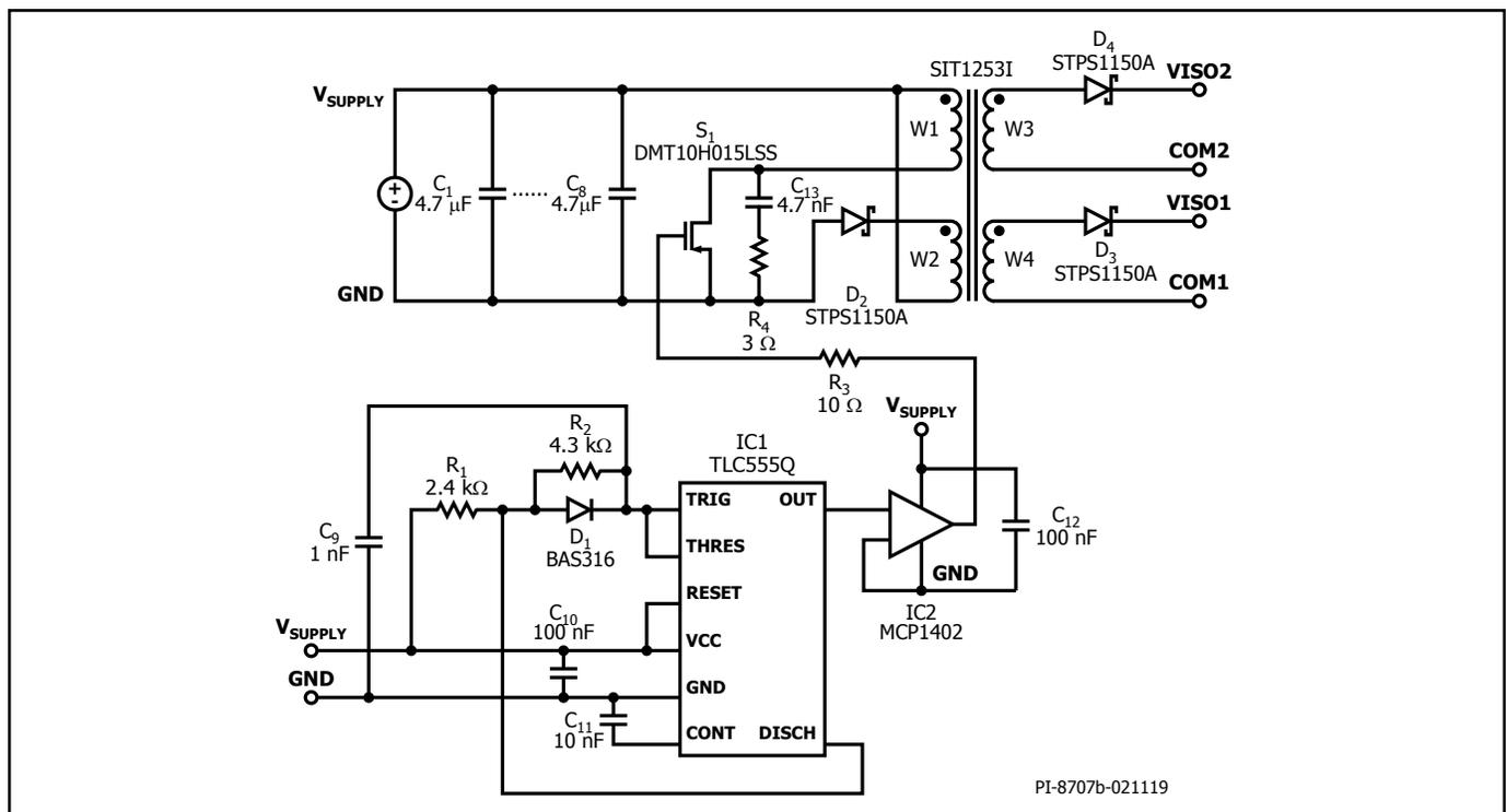
Figure 4. Application Example SIT1253I with 5 V Supply Voltage.
