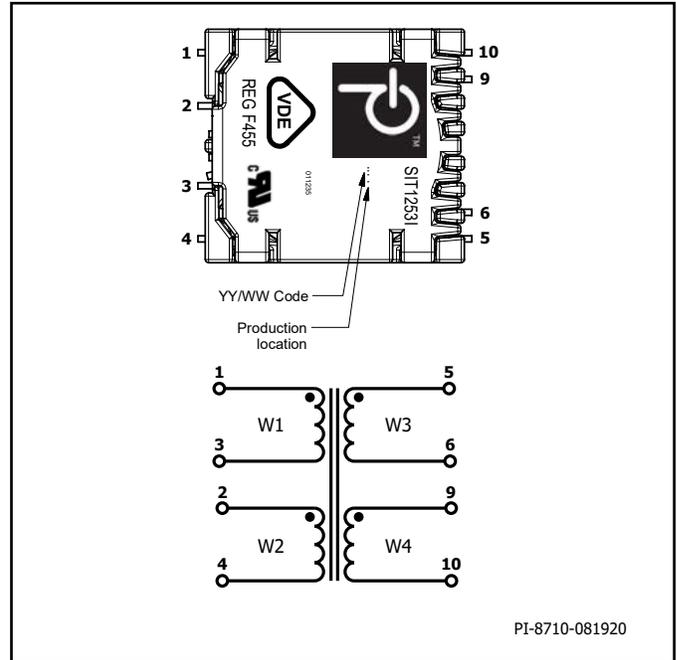
Figure 3. Top View Footprint and Pin Assignment.
