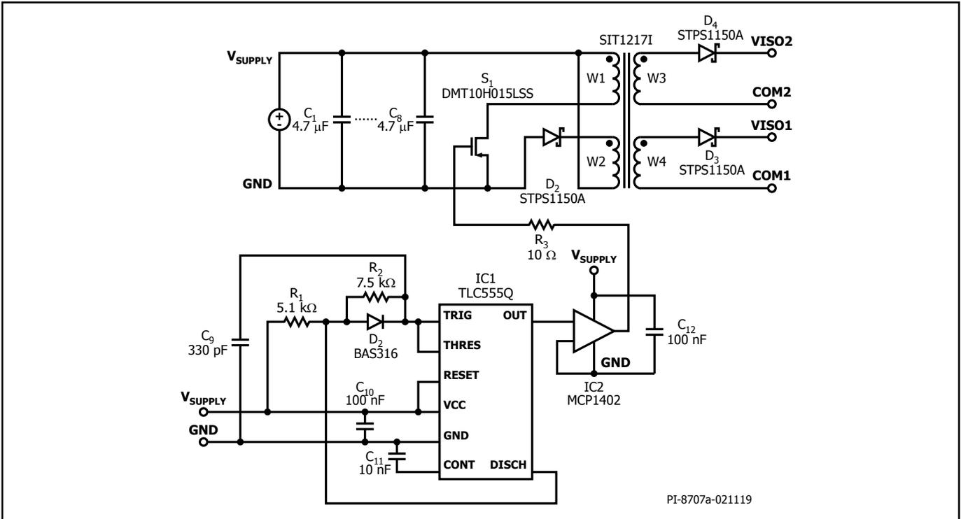
Figure 5. Application Example SIT1217I with 15 V Supply Voltage.
