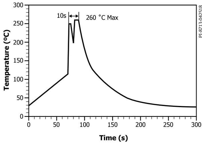
Figure 13. Solder Profiles According to BS CECC 00802 / Wave.
