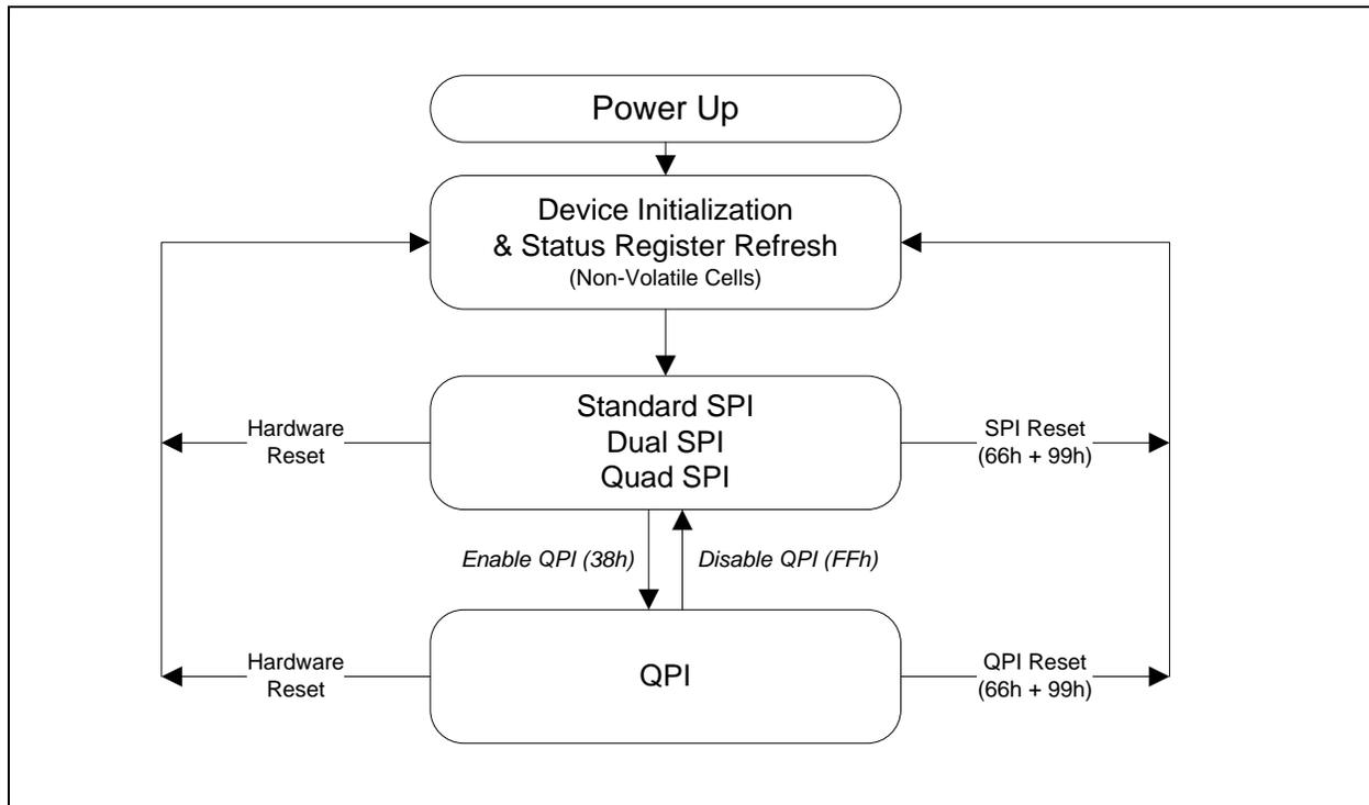
Figure 3. W25Q128JW Serial Flash Memory Operation Diagram
