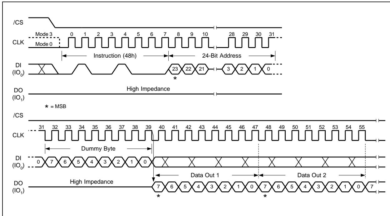
Figure 47. Read Security Registers Instruction (SPI Mode only)
