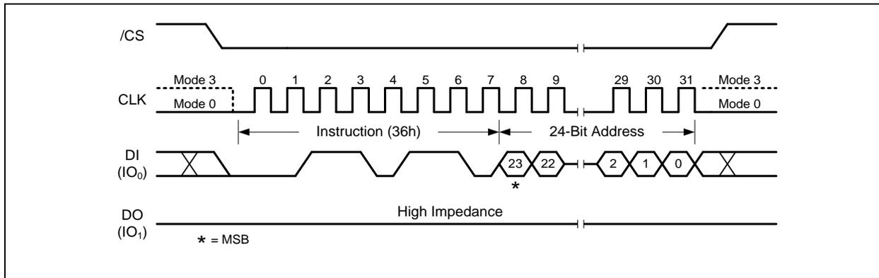
Figure 53a. Individual Block/Sector Lock Instruction (SPI Mode)
