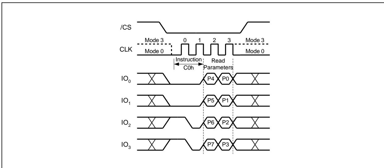
Figure 48. Set Read Parameters Instruction (QPI Mode only)
