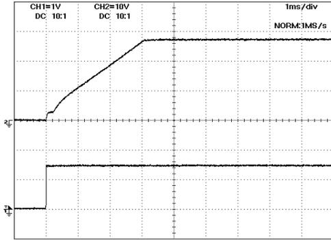
Plot 1 Start-up response at max output voltage 1mA load
