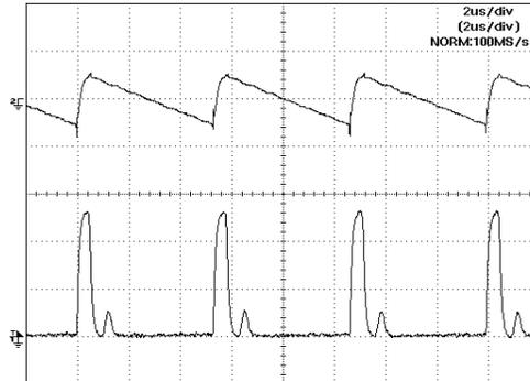
Plot 4 Operating waveforms at max output voltage 10mA load
