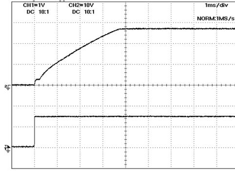
Plot 2 Start-up response at max output voltage 5mA load
