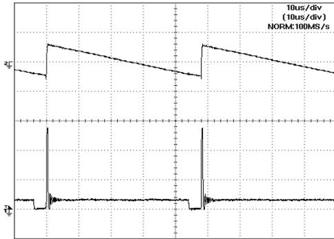
Plot 3 Operating waveforms at max output voltage 1mA load
