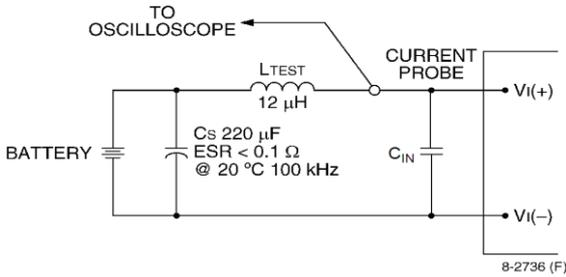
Note: Measure the input reflected-ripple current with a simulated source inductance (LTEST) of 12 µH. Capacitor CS offsets possible battery impedance. Measure the current, as shown above.
