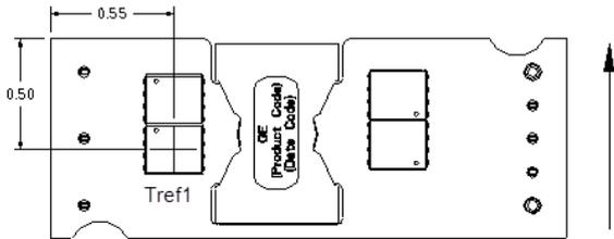
Figure 17. Case ( $T_{REF}$ ) Temperature Measurement Location (top view).
