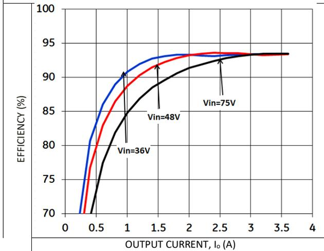
Figure 1. Converter Efficiency versus Output Current.
