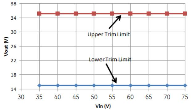
**Figure 12. Output Voltage Trim Limits vs. Input Voltage.**
