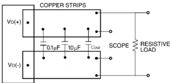
Note: Use a Cout (470 µF Low ESR aluminum or tantalum capacitor typical), a 0.1 µF ceramic capacitor and a 10 µF ceramic capacitor, and Scope measurement should be made using a BNC socket. Position the load between 51 mm and 76 mm (2 in. and 3 in.) from the module.
