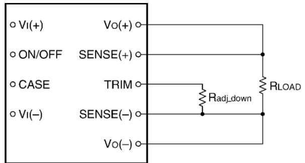
**Figure 13. Circuit Configuration to Decrease Output Voltage.**
