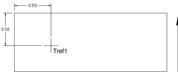
Figure 18. Case ( $T_{REF}$ ) Temperature Measurement Location (top view).
