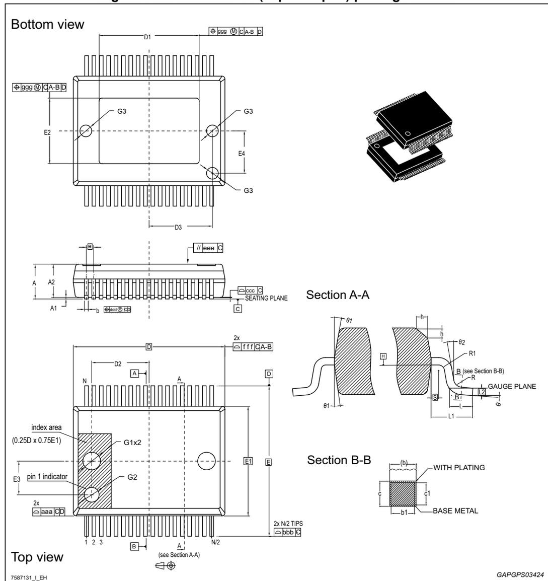
Table 33. PowerSSO-36 exposed pad (D1 and E2 use the option variation B) package mechanical data
