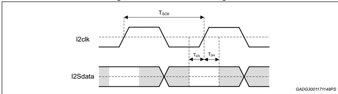
Figure 68. I<sup>2</sup>S clock transition timings
