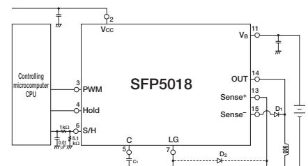
\* Use a Schottky Di for D2 when the Sense+ terminal is lower than the abs. max. rated voltage (-0.8V)
