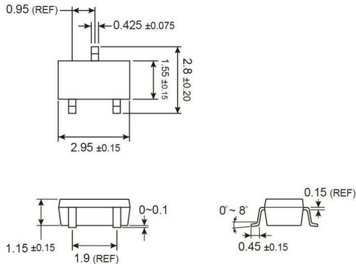
**SUGGESTED PAD LAYOUT** (Unit: Millimeters)
