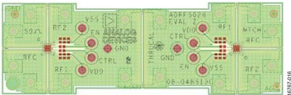
Figure 16. Evaluation Board Layout
