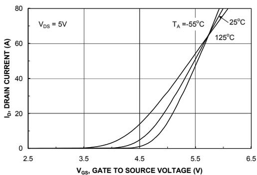
Figure 5. Transfer Characteristics.
