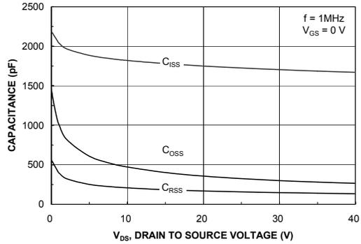
**Figure 8. Capacitance Characteristics.**
