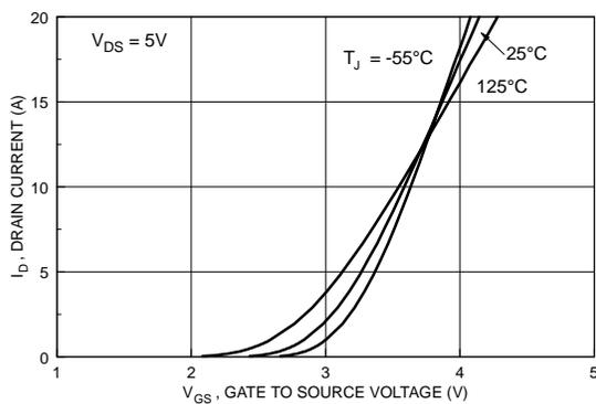
Figure 5. Transfer Characteristics.
