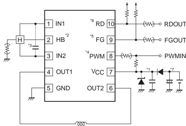
\*1 < Capacitor for power stabilization >
