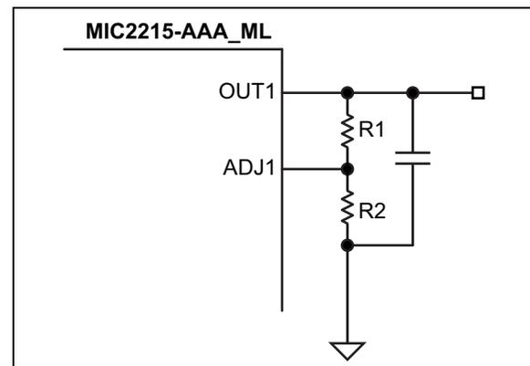
**FIGURE 5-1:** Adjustable Output.
