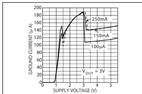
**FIGURE 2-23:** Ground Current vs. Supply Voltage for LDO 1.
