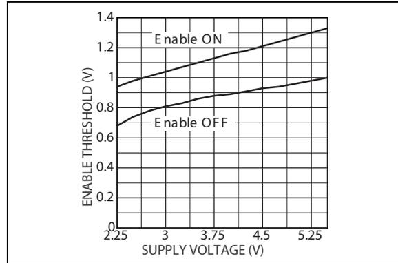
**FIGURE 2-10:** *Enable Threshold vs. Supply Voltage for LDO 1.*
