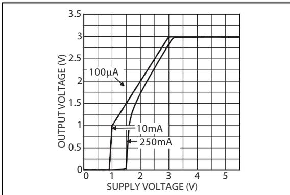
**FIGURE 2-27:** Output Voltage vs. Supply Voltage for LDO 2.
