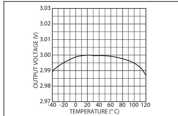
**FIGURE 2-5:** Output Voltage vs. Temperature for LDO 2.
