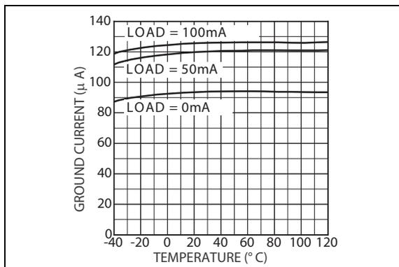
**FIGURE 2-3:** Ground Current vs. Temperature for LDO 3.
