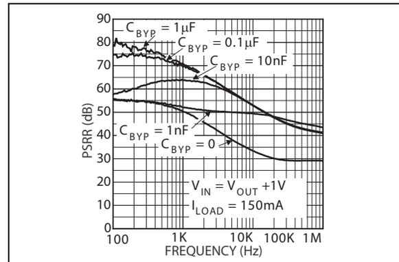
**FIGURE 2-30:** Power Supply Rejection Ratio vs.  $C_{BYPASS}$ .
