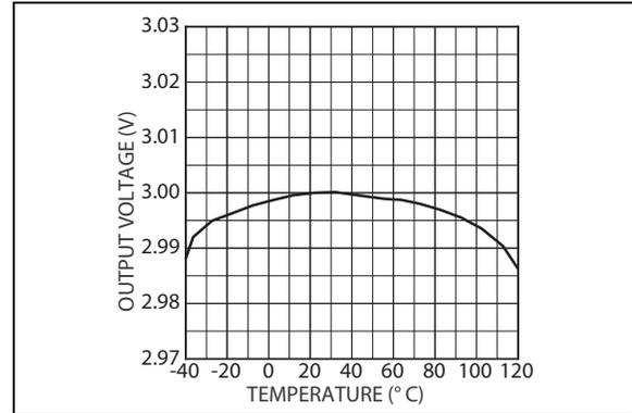
**FIGURE 2-4:** Output Voltage vs. Temperature for LDO 1.
