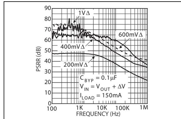
**FIGURE 2-29:** Power Supply Rejection Ratio,  $3V_{OUT}$ .
