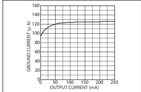
**FIGURE 2-16:** Ground Current vs. Load Current for LDO 3.
