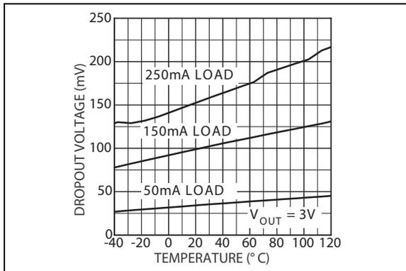
**FIGURE 2-9:** *Dropout Voltage vs. Temperature for LDO 3.*
