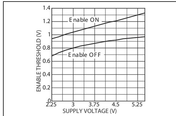
**FIGURE 2-11:** *Enable Threshold vs. Supply Voltage for LDO 2.*
