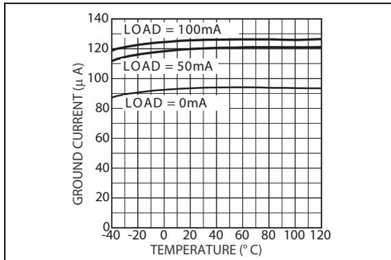
**FIGURE 2-2:** Ground Current vs. Temperature for LDO 2.
