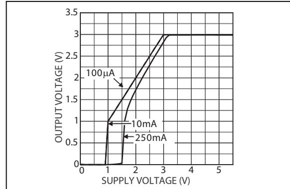
**FIGURE 2-28:** Output Voltage vs. Supply Voltage for LDO 3.
