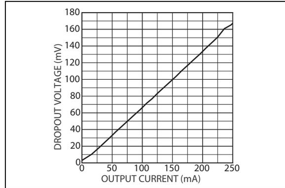
**FIGURE 2-22:** Dropout Voltage vs. Output Current for LDO 3.
