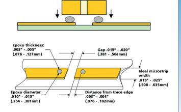
4. After the reflow step is completed, inspect joint for voids or excess flux and non-reflowed solder balls that can degrade performance or cause shorts across the gaps. Proper cleaning after the reflow process is crucial to avoiding performance degradation and discovering poor solder joints. Isopropanol and Methanol are both safe to use with soldered Milli-Caps®.
