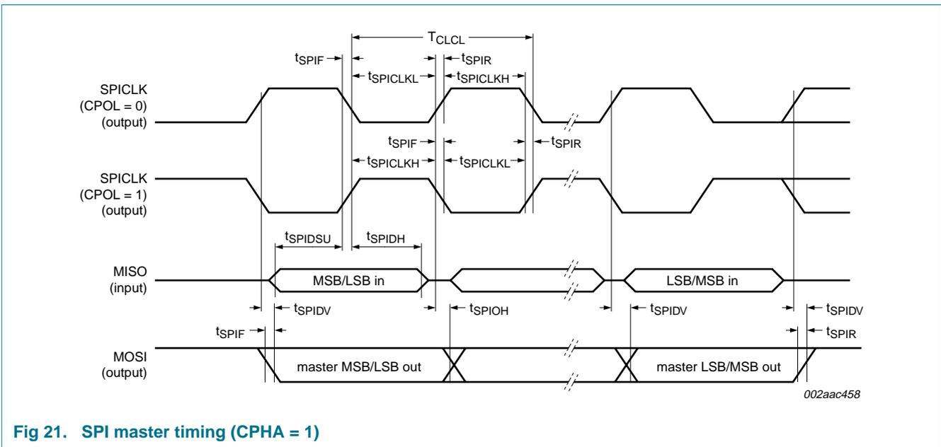
Fig 21. SPI master timing (CPHA = 1)
