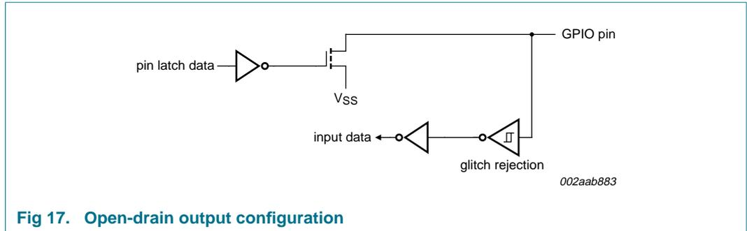
Fig 17. Open-drain output configuration
