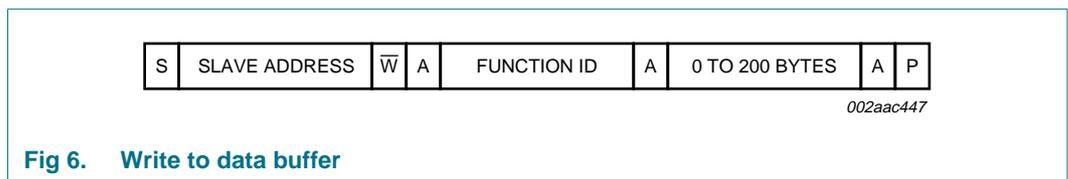
Fig 6. Write to data buffer
