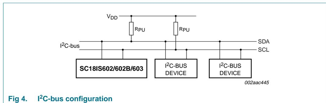
Fig 4. I<sup>2</sup>C-bus configuration
