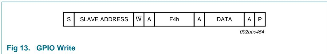
**Fig 13. GPIO Write**
