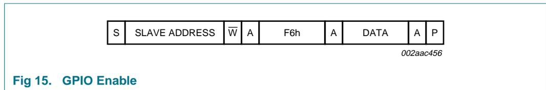
Fig 15. GPIO Enable
