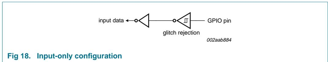
Fig 18. Input-only configuration
