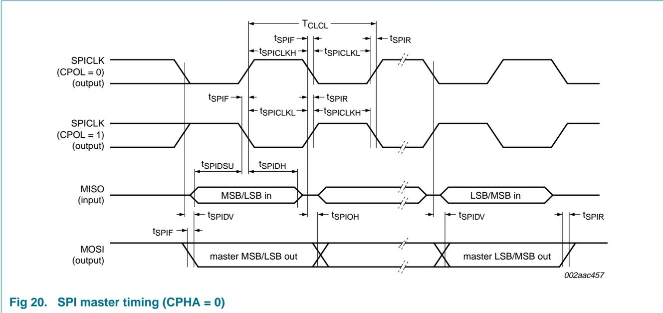
Fig 20. SPI master timing (CPHA = 0)
