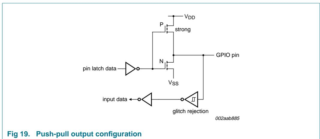
Fig 19. Push-pull output configuration
