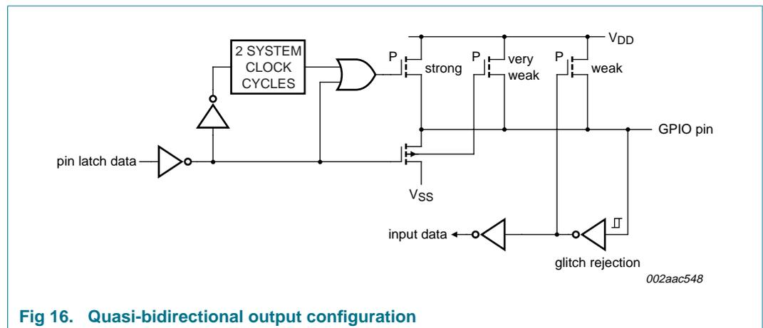
**Fig 16. Quasi-bidirectional output configuration**
