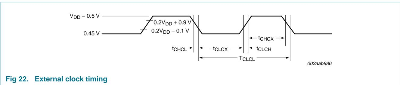
Fig 22. External clock timing
