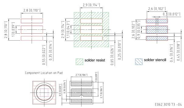
For superior solder joint connectivity results we recommend soldering under standard nitrogen atmosphere.
