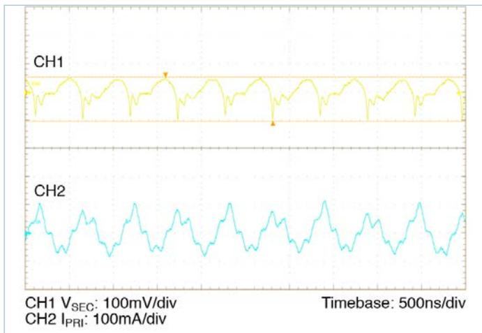
Figure 14 — Full-load secondary voltage and primary current ripple,  $2700\mu F C_{PRI\_IN\_EXT}$ ; no external  $C_{SEC\_OUT\_EXT}$ .
