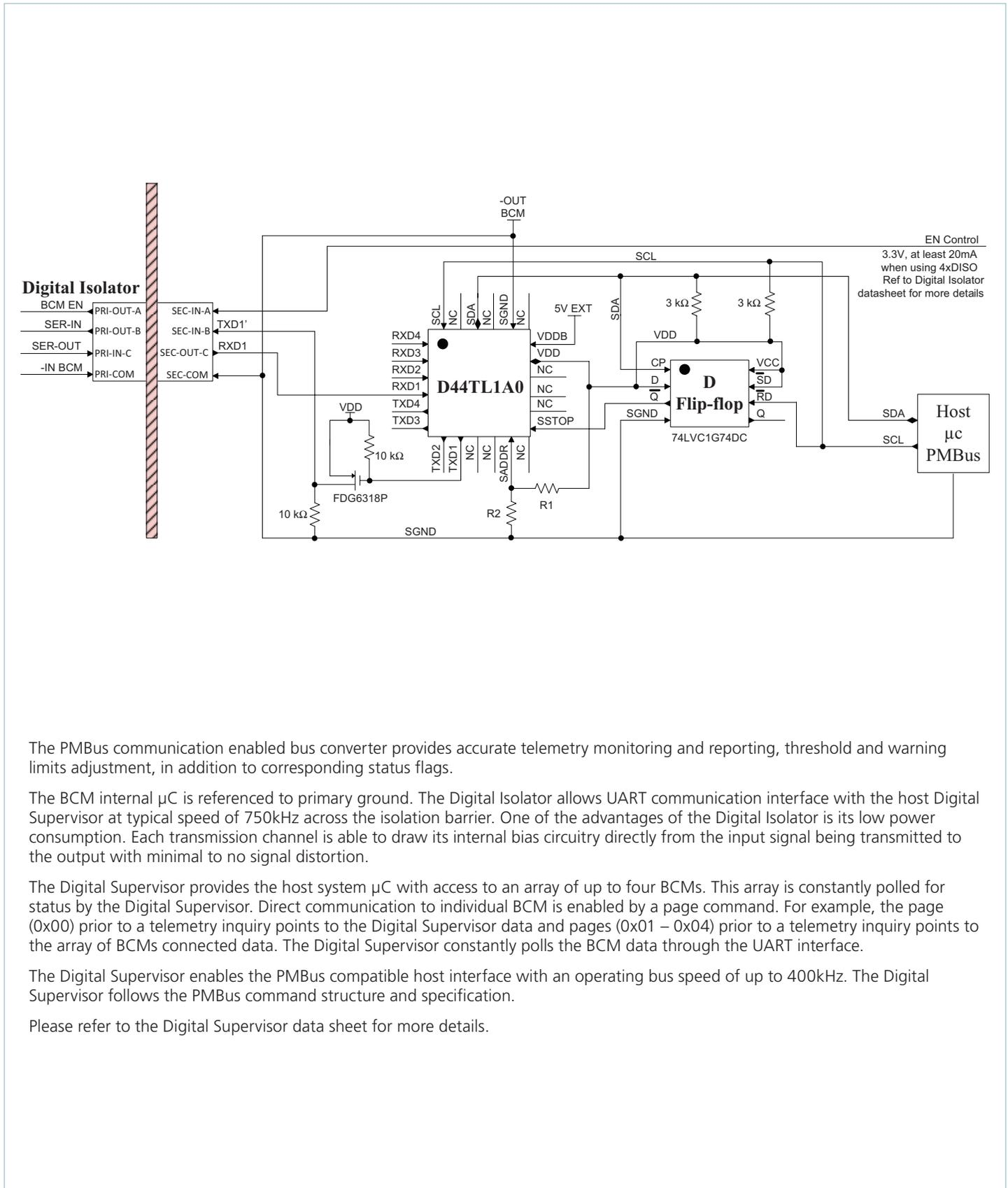
The PMBus communication enabled bus converter provides accurate telemetry monitoring and reporting, threshold and warning limits adjustment, in addition to corresponding status flags.
