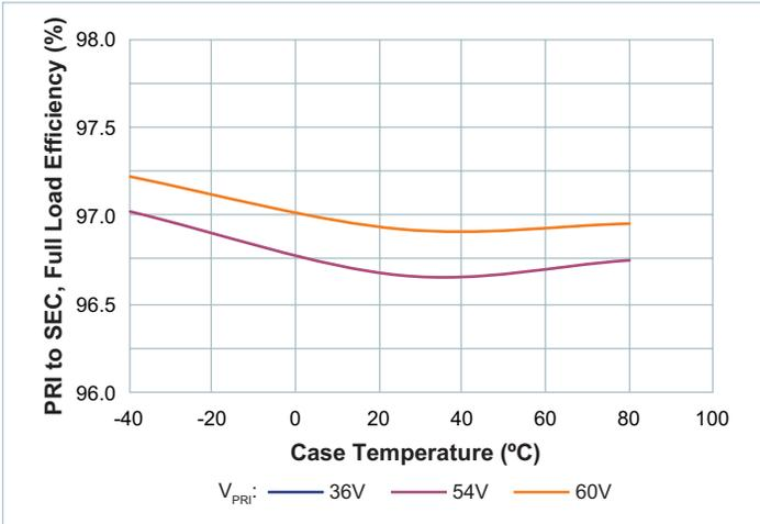
Figure 5 — Full-load efficiency vs. temperature;  $V_{PRI\_DC}$
