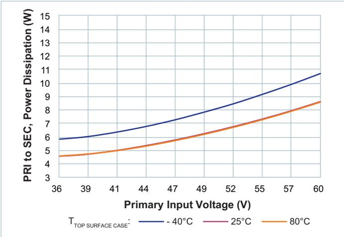
Figure 4 — No-load power dissipation vs.  $V_{PRI\_DC}$
