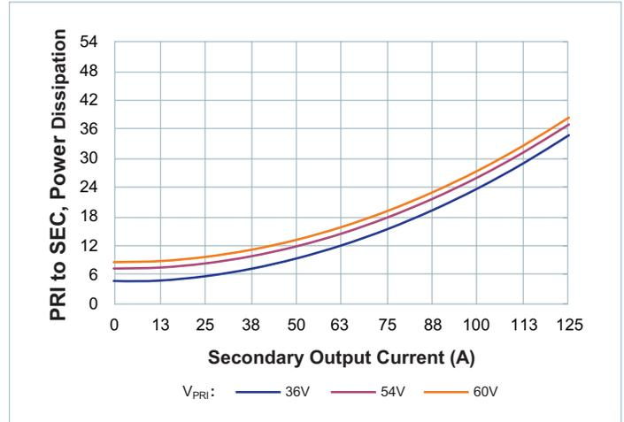
Figure 11 — Power dissipation at  $T_{CASE} = 80^{\circ}C$
