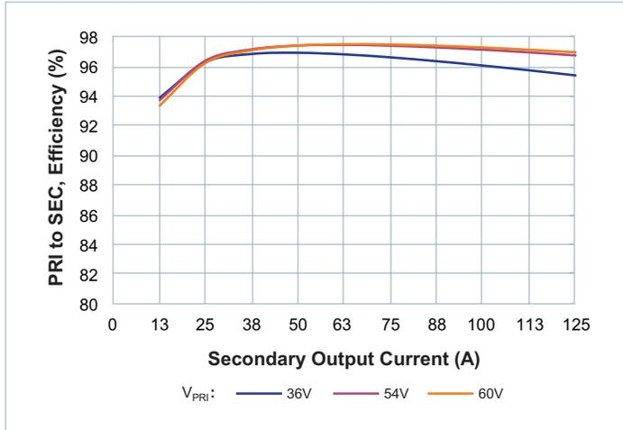
Figure 10 — Efficiency at  $T_{CASE} = 80^{\circ}C$
