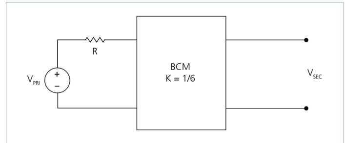
Figure 20 — K = 1/6 BCM with series primary resistor
