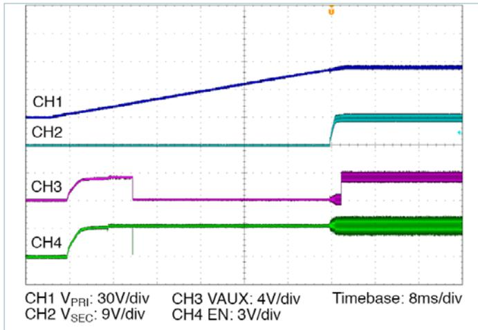
Figure 17 — Start up from application of V<sub>PRI\_DC</sub> = 54V,
