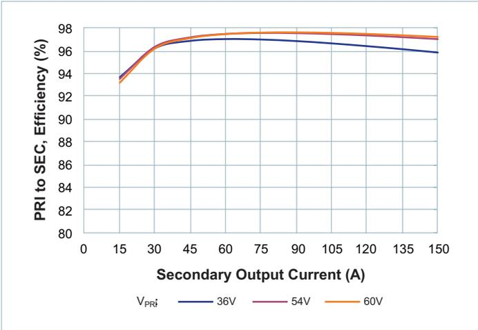
Figure 6 — Efficiency at  $T_{CASE} = -40^\circ C$
