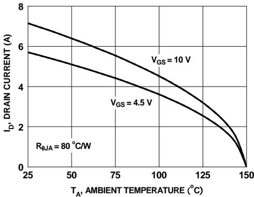
**Figure 9. Maximum Continuous Drain Current vs Ambient Temperature**
