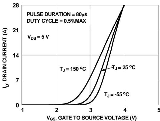
**Figure 5. Transfer Characteristics**
