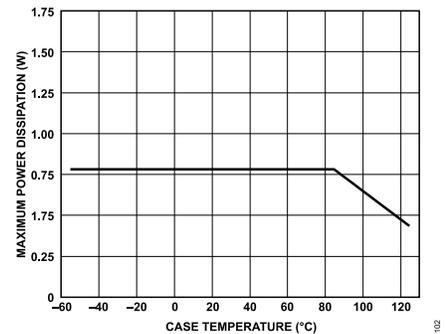
**Figure 2. Maximum Power Dissipation vs. Case Temperature**
