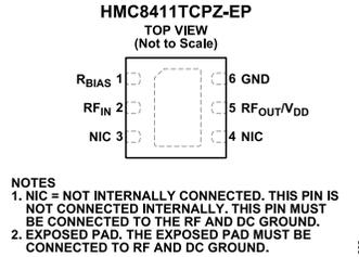
Figure 3. Pin Configuration
