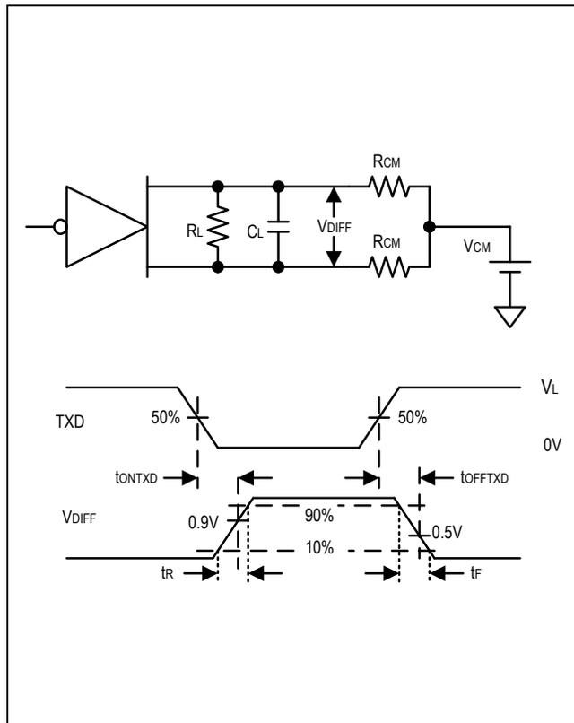
Figure 1. Transmitter Test Circuit and Timing Diagram
