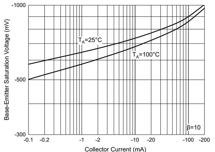
Fig. 5 - Base-Emitter Voltage Characteristics
