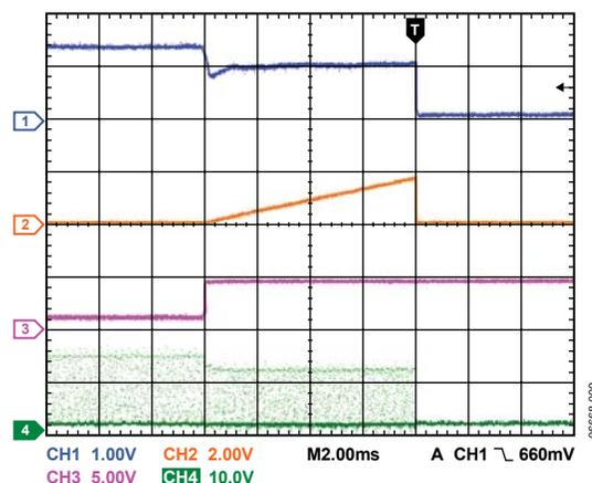
Figure 9. Overcurrent Latch-Off Waveforms
