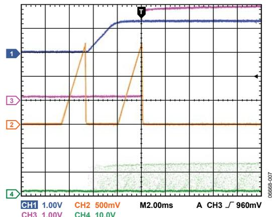
Figure 8. Typical Start-up Waveforms
