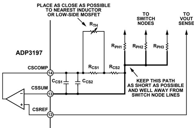
Figure 11. Temperature Compensation Circuit Values
