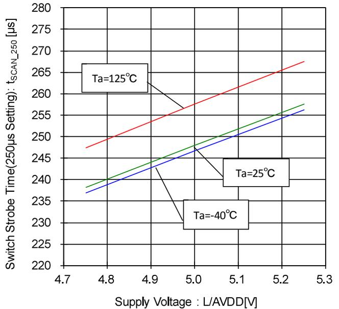
Figure 116. Switch Strobe Time- Voltage Characteristic (250µs Setting)
