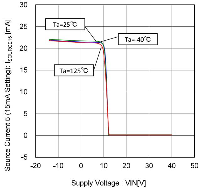
Figure 66. Source Current 5- Voltage Characteristic (15mA Setting)
