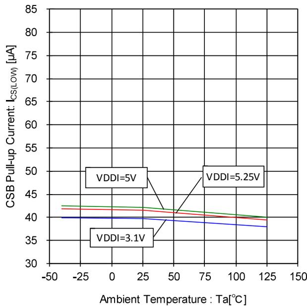
Figure 83. CSB Pull-up Current- Temperature Characteristic (CSB=0V)
