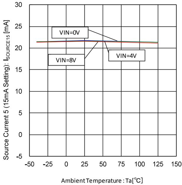
Figure 65. Source Current 5- Temperature Characteristic (15mA Setting)
