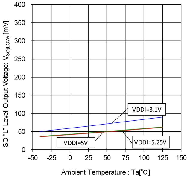
Figure 91. SO "L" Level Output Voltage- Temperature Characteristic (I<sub>SINK</sub>=1.6mA)
