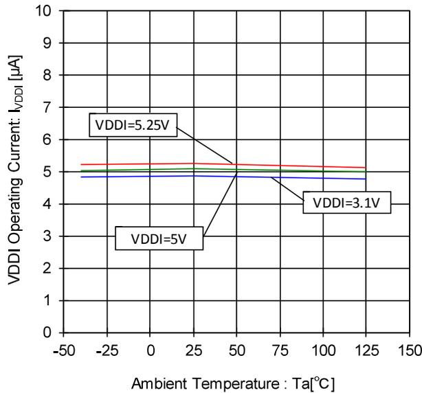
Figure 27. VDDI Operating Current- Temperature Characteristic (INTB="H", CSB="H")
