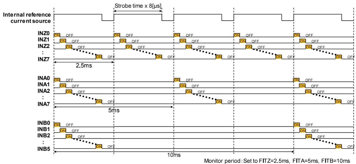
Figure 15. Sequential Monitoring by Power Supply System Example
