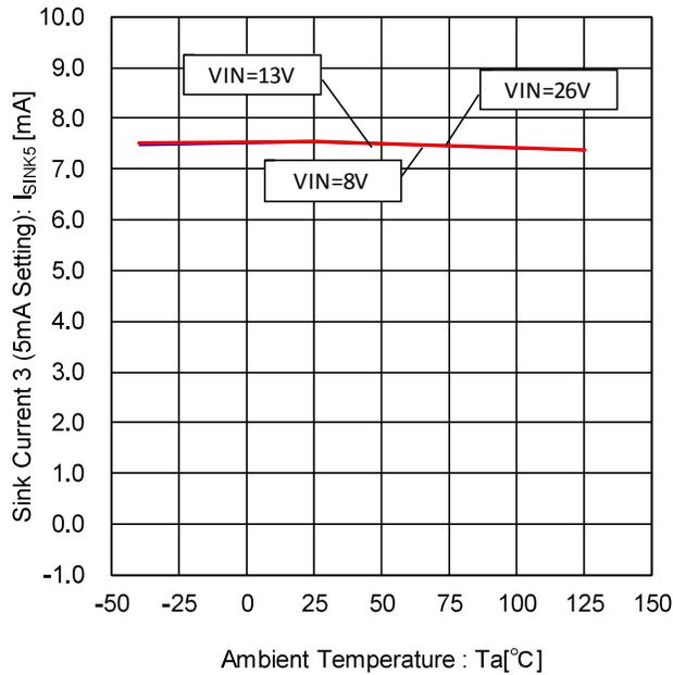
Figure 53. Sink Current 3- Temperature Characteristic (5mA Setting)
