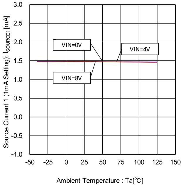
Figure 33. Source Current 1- Temperature Characteristic (1mA Setting)
