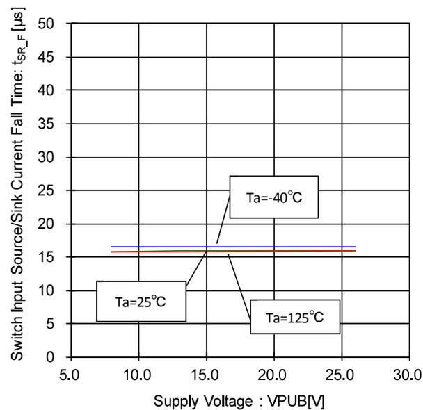
Figure 120. Switch Input Source/Sink Current Fall Time-Voltage Characteristic
