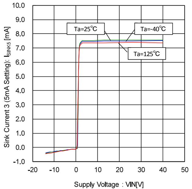
Figure 54. Sink Current 3- Voltage Characteristic (5mA Setting)
