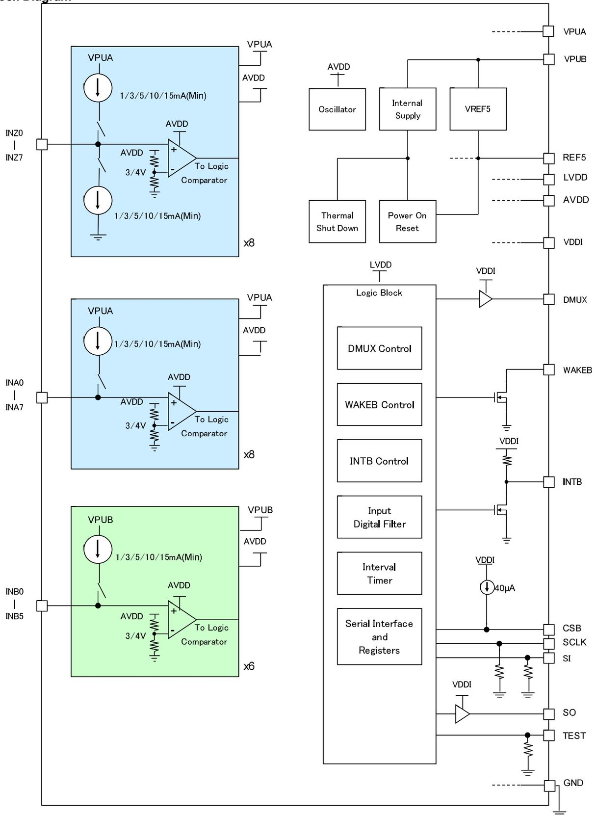
Figure 3. Block Diagram
