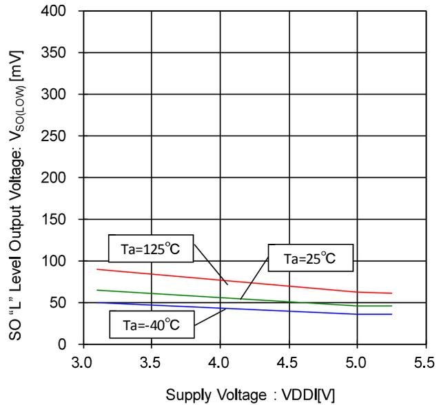
Figure 92. SO "L" Level Output Voltage- Voltage Characteristic (I<sub>SINK</sub> =1.6mA)
