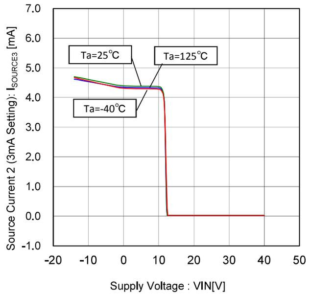
Figure 42. Source Current 2- Voltage Characteristic (3mA Setting)
