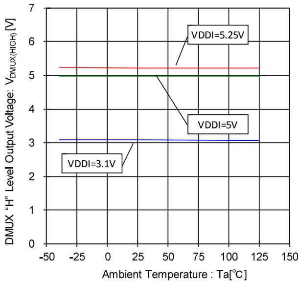
Figure 95. DMUX "H" Level Output Voltage- Temperature Characteristic (I<sub>SOURCE</sub>=200μA)
