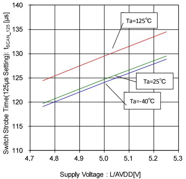
Figure 112. Switch Strobe Time- Voltage Characteristic (125µs Setting)
