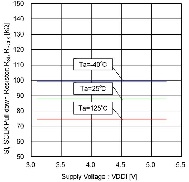
Figure 86. SI, SCLK Pull-down Resistor- Voltage Characteristic
