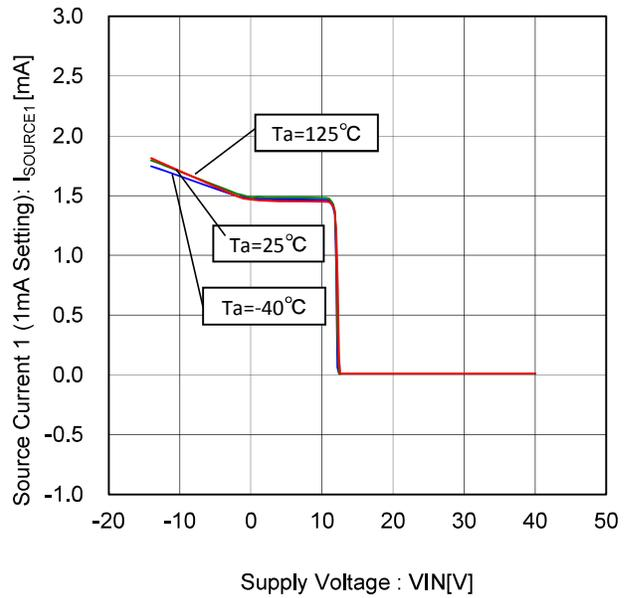
Figure 34. Source Current 1- Voltage Characteristic (1mA Setting)
