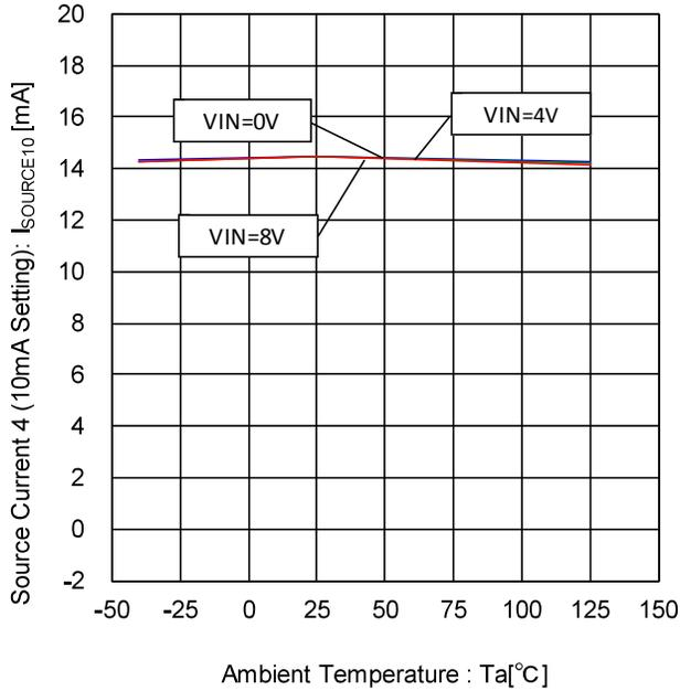
Figure 57. Source Current 4- Temperature Characteristic (10mA Setting)
