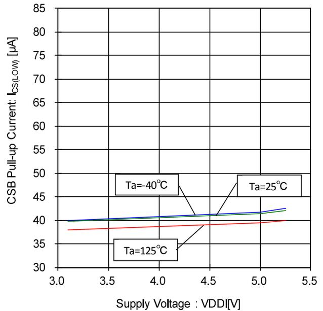
Figure 84. CSB Pull-up Current- Voltage Characteristic (CSB=0V)
