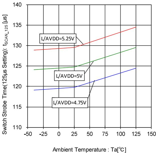
Figure 111. Switch Strobe Time- Temperature Characteristic (125µs Setting)
