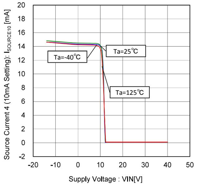
Figure 58. Source Current 4- Voltage Characteristic (10mA Setting)
