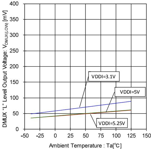
Figure 97. DMUX "L" Level Output Voltage- Temperature Characteristic (I<sub>SINK</sub>=1.6mA)
