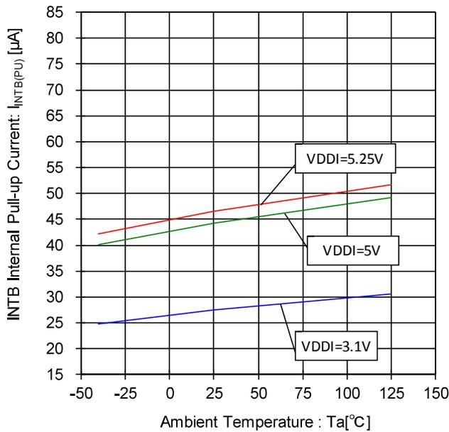
Figure 99. INTB Internal Pull-up Current- Temperature Characteristic
