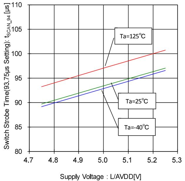
Figure 110. Switch Strobe Time- Voltage Characteristic (93.75µs Setting)
