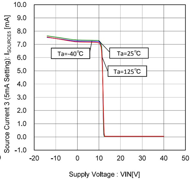
Figure 50. Source Current 3- Voltage Characteristic (5mA Setting)
