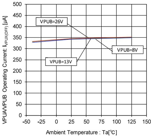
Figure 23. V\_PUA/V\_PUB Operating Current - Temperature Characteristic
