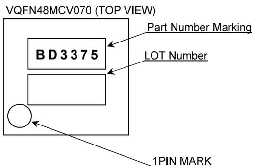
Figure 125. Marking Diagrams
