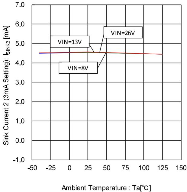
Figure 45. Sink Current 2- Temperature Characteristic (3mA Setting)
