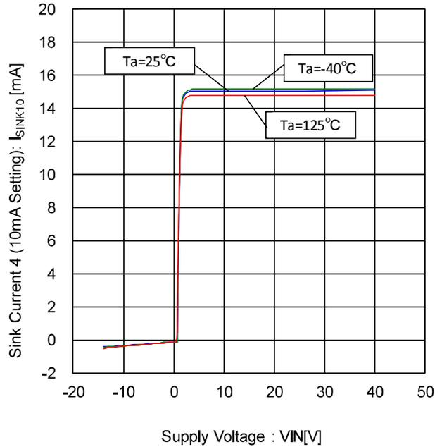
Figure 62. Sink Current 4- Voltage Characteristic (10mA Setting)
