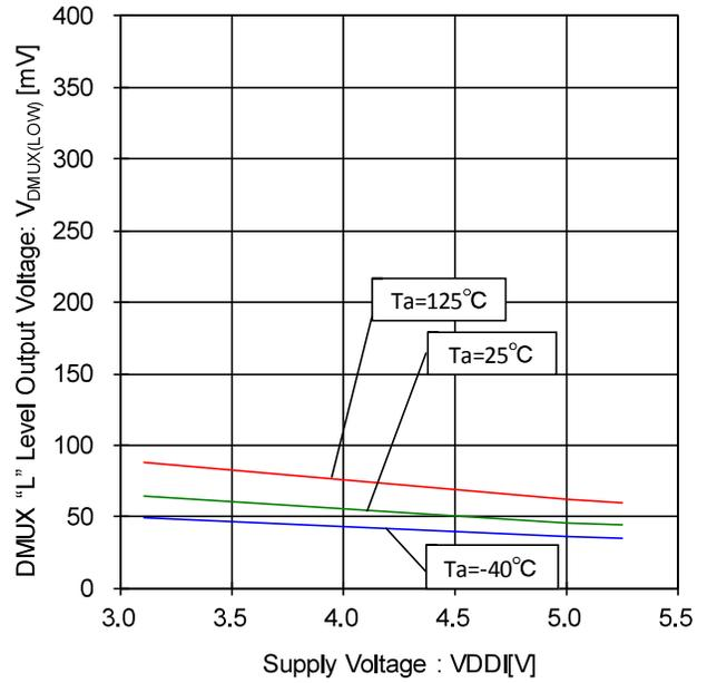
Figure 98. DMUX "L" Level Output Voltage- Voltage Characteristic (I<sub>SINK</sub>=1.6mA)
