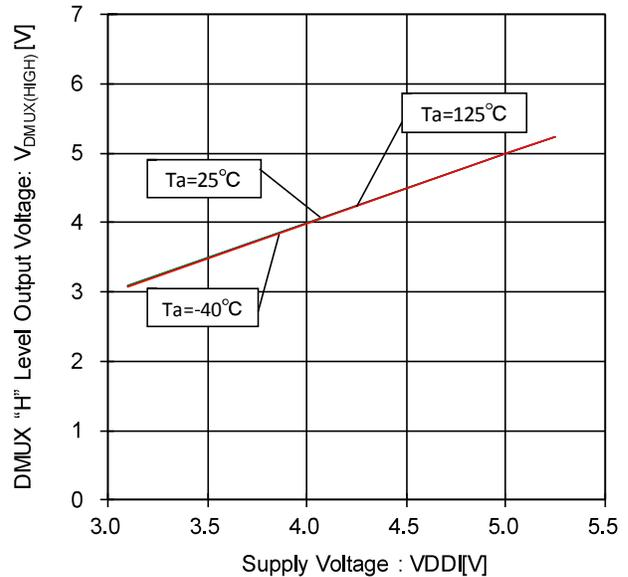
Figure 96. DMUX "H" Level Output Voltage- Voltage Characteristic (I<sub>SOURCE</sub>=200μA)
