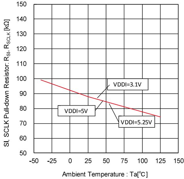
Figure 85. SI, SCLK Pull-down Resistor- Temperature Characteristic
