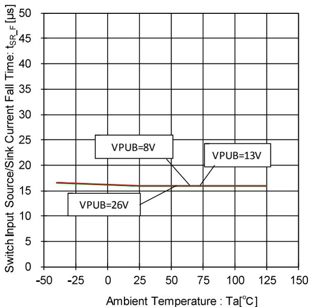
Figure 119. Switch Input Source/Sink Current Fall Time-Temperature Characteristic
