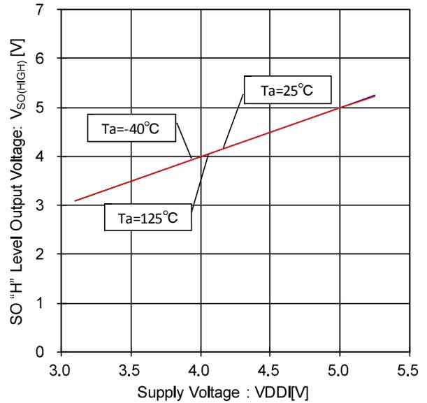
Figure 90. SO "H" Level Output Voltage- Voltage Characteristic (I<sub>SOURCE</sub>=200μA)
