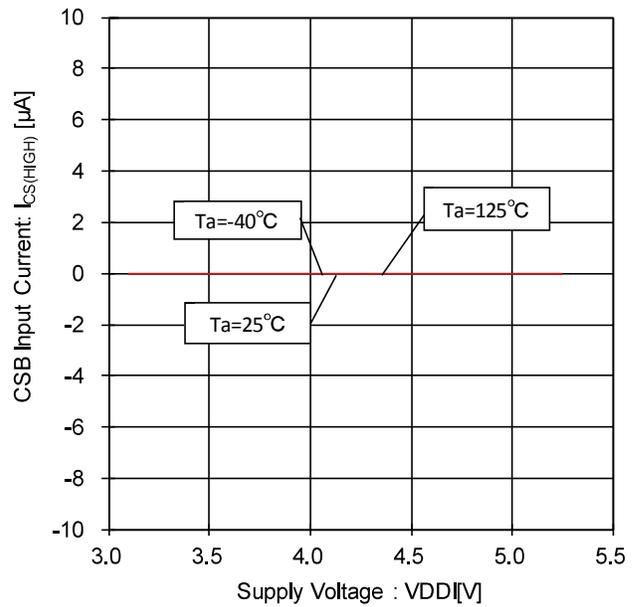
Figure 82. CSB Input Current- Voltage Characteristic (CSB=VDDI)
