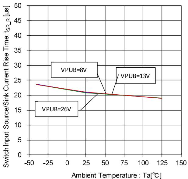
Figure 117. Switch Input Source/Sink Current Rise Time-Temperature Characteristic
