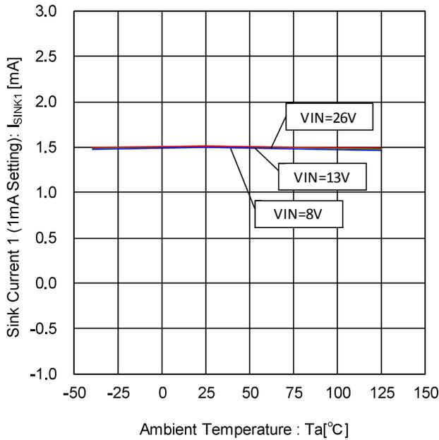
Figure 37. Sink Current 1- Temperature Characteristic (1mA Setting)
