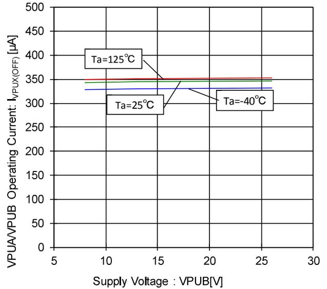
Figure 24. V\_PUA/V\_PUB Operating Current - Voltage Characteristic
