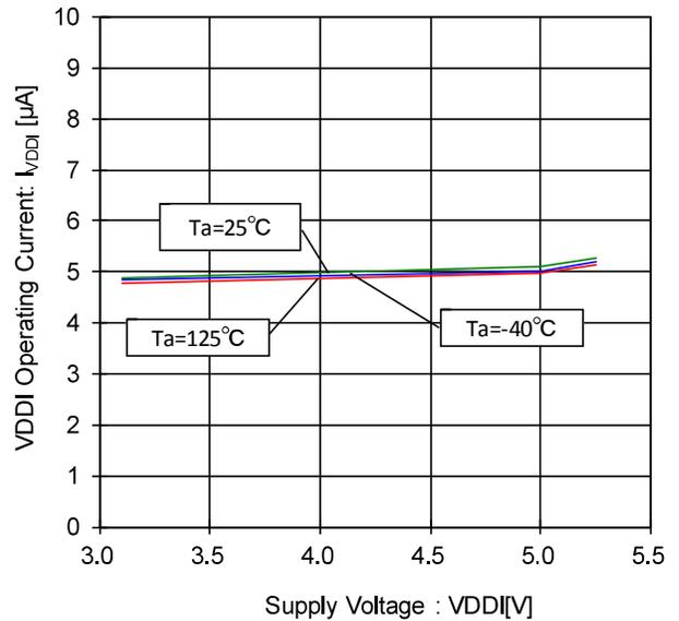
Figure 28. VDDI Operating Current- Voltage Characteristic (INTB="H", CSB="H")
