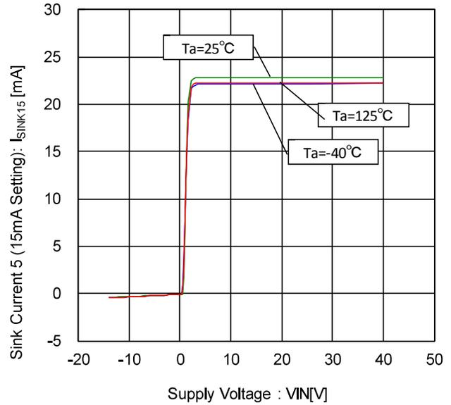
Figure 70. Sink Current 5- Voltage Characteristic (15mA Setting)
