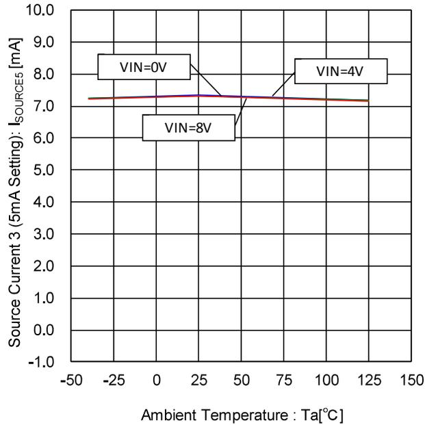
Figure 49. Source Current 3- Temperature Characteristic (5mA Setting)
