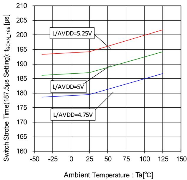
Figure 113. Switch Strobe Time- Temperature Characteristic (187.5µsSetting)
