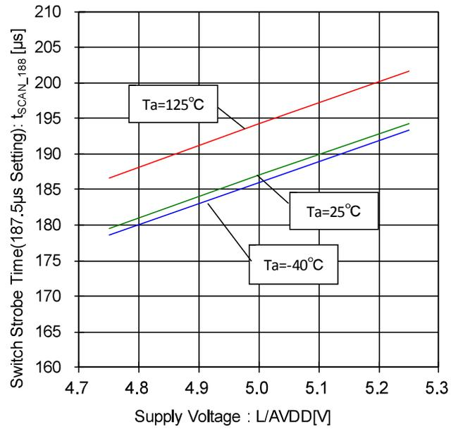
Figure 114. Switch Strobe Time- Voltage Characteristic (187.5µsSetting)
