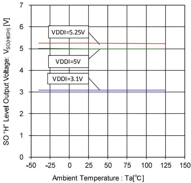
Figure 89. SO "H" Level Output Voltage- Temperature Characteristic (I<sub>SOURCE</sub>=200μA)
