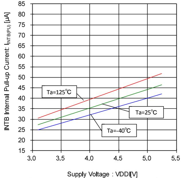
Figure 100. INTB Internal Pull-up Current- Voltage Characteristic
