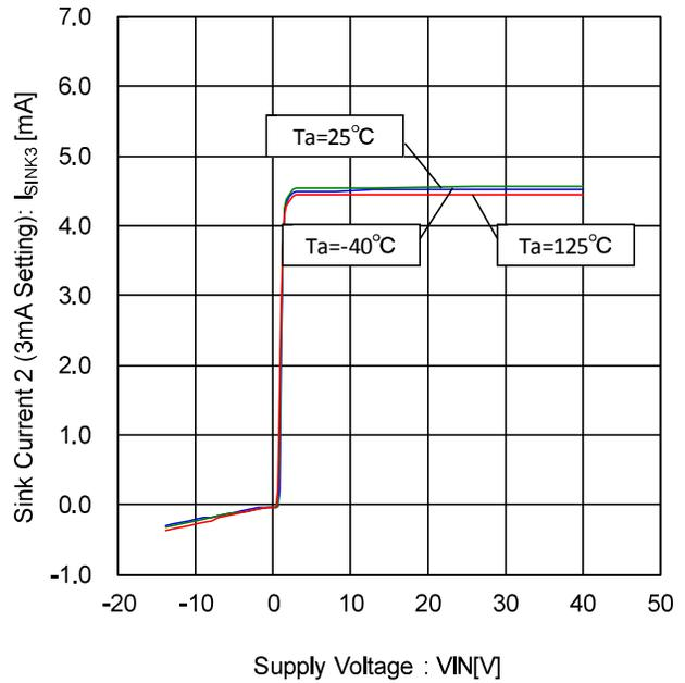
Figure 46. Sink Current 2- Voltage Characteristic (3mA Setting)
