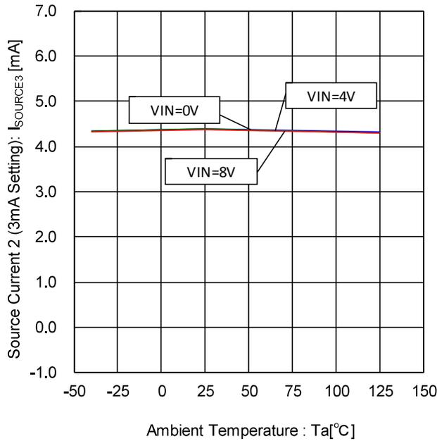
Figure 41. Source Current 2- Temperature Characteristic (3mA Setting)
