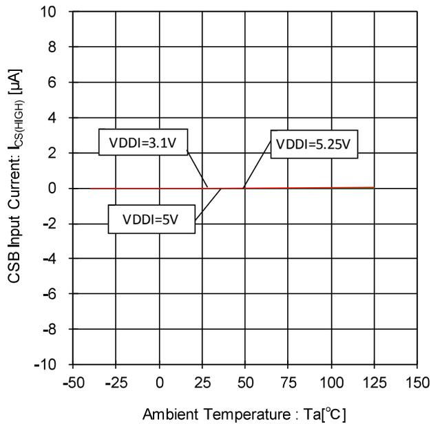
Figure 81. CSB Input Current- Temperature Characteristic (CSB=VDDI)
