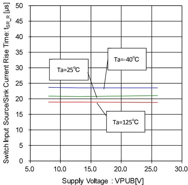
Figure 118. Switch Input Source/Sink Current Rise Time-Voltage Characteristic
