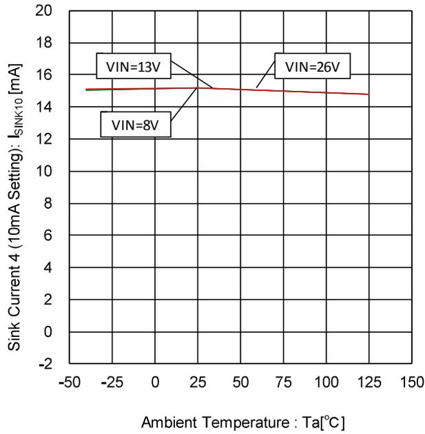
Figure 61. Sink Current 4- Temperature Characteristic (10mA Setting)
