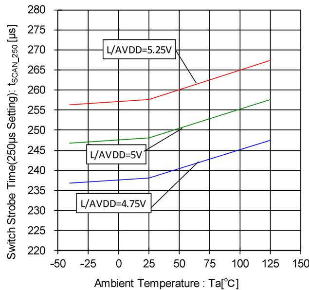
Figure 115. Switch Strobe Time- Temperature Characteristic (250µs Setting)
