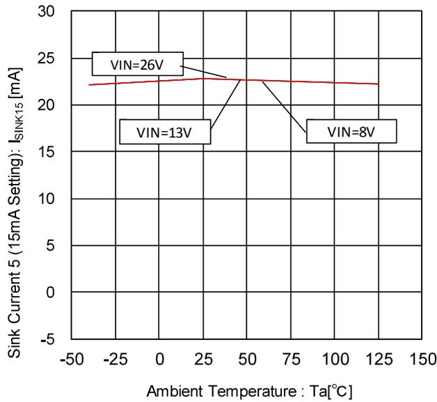
Figure 69. Sink Current 5- Temperature Characteristic (15mA Setting)
