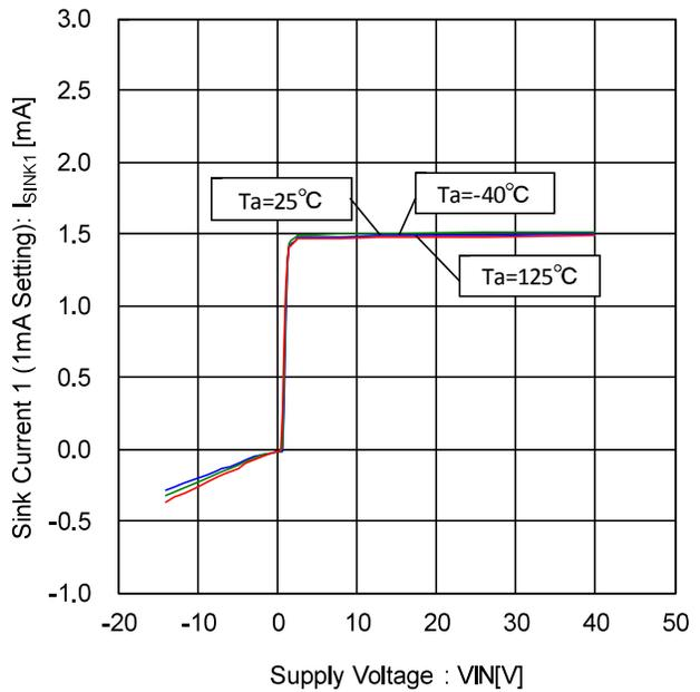
Figure 38. Sink Current 1- Voltage Characteristic (1mA Setting)
