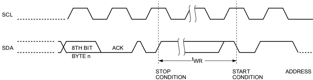
**Figure 4. Start/Stop Timing**
