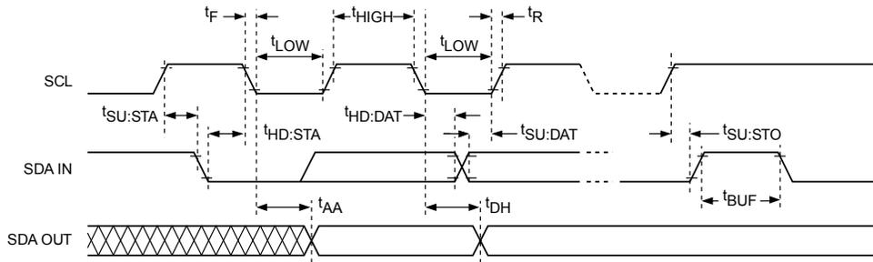
**Figure 3. Write Cycle Timing**
