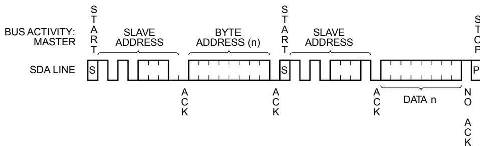
**Figure 11. Sequential Read Timing**
