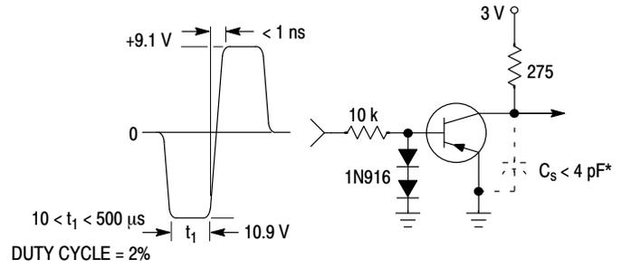
Figure 20. Storage and Fall Time Equivalent Test Circuit
