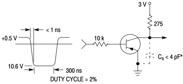
Figure 19. Delay and Rise Time Equivalent Test Circuit
