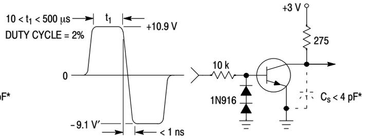
Figure 2. Storage and Fall Time Equivalent Test Circuit
