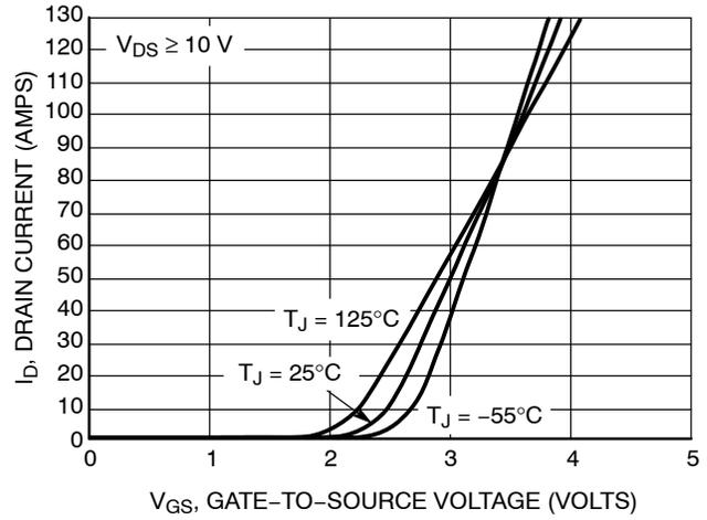
Figure 2. Transfer Characteristics
