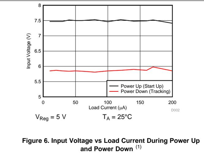
(1) **Figure 5** shows the dropout operation during low input conditions. **Figure 6** shows the following plots:
