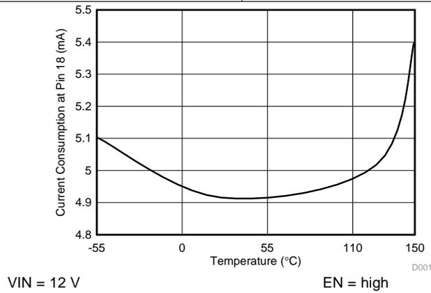
**Figure 9. Current Consumption With Temperature**
