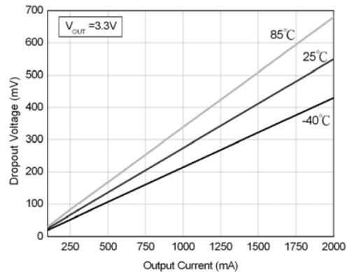
Fig. 11: Dropout Voltage at  $V_{OUT} = 3.3V$
