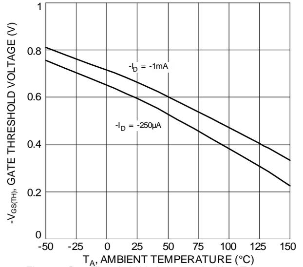
Figure 8 Gate Threshold Variation vs. Ambient Temperature
