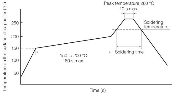
Soldering temperature and Soldering time
